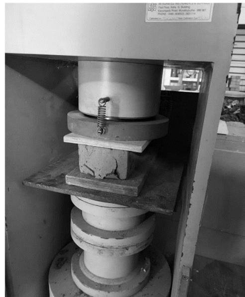
Fig. 6 Compressive Strength Test of Unfired Thamarachal Brick
