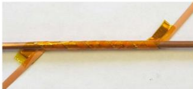
Figure 6.6 A 3 mm wide superconducting tape containing a 30 \mu\text{m} thick substrate wound onto a 2.8 mm diameter former. A 3 mm wide copper tape is wound in parallel to the superconducting tape to ensure a constant winding angle close to 45. [[D C van der lan et.al]
