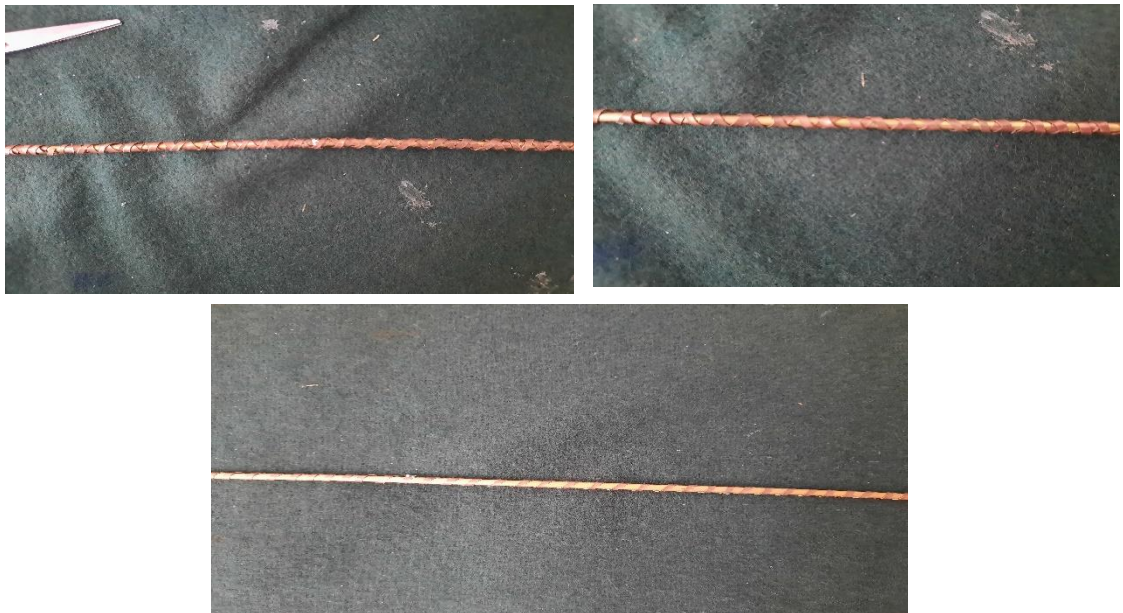
Figure 6.8 Arrangement of CORC cable structures -2 mm copper sheet winded on 3 mm diameter brass rod at 45 degree
