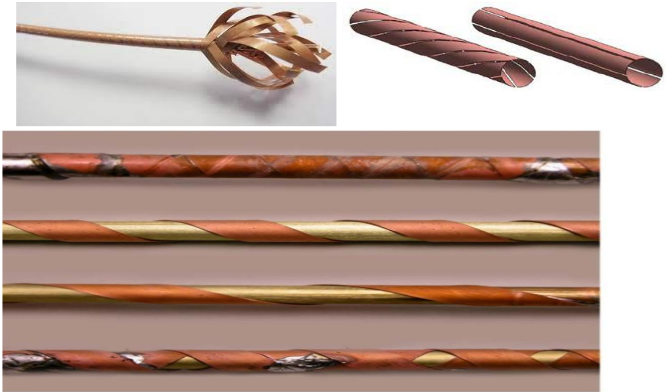
Figure 6.7 CORC cable arrangement a) Original arrangement b) Orientation for numerical studies [M solovyov et.al] c)Arrangement for experimental studies[D C van der lan et.al]
