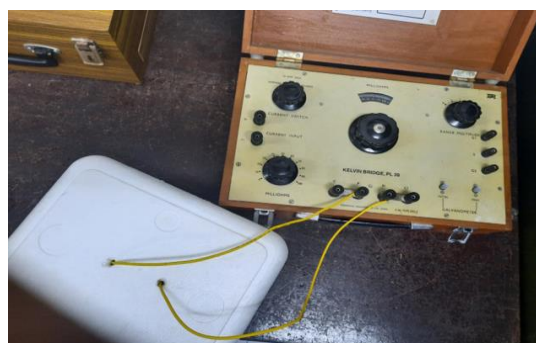
Figure 5.4 Connections of specimen at LN2 temperature to kelvins double bridge
