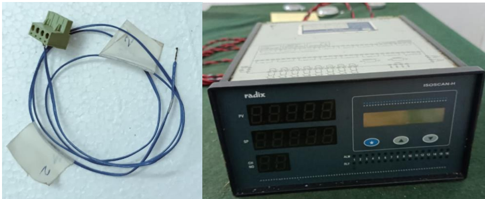
Fig. 6.1 (a) Type T Thermocouple (b) Temperature indicator
