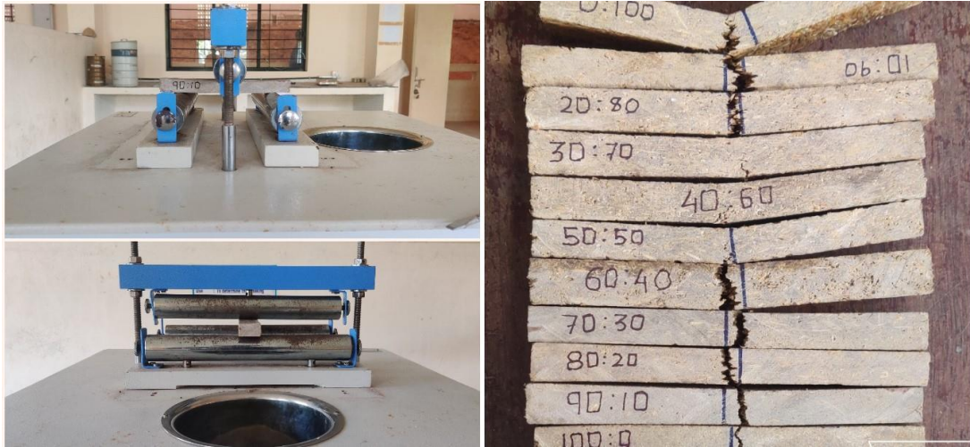
Fig. 3.15: 3 Point flexural Testing machine for flexural strength calculation.
