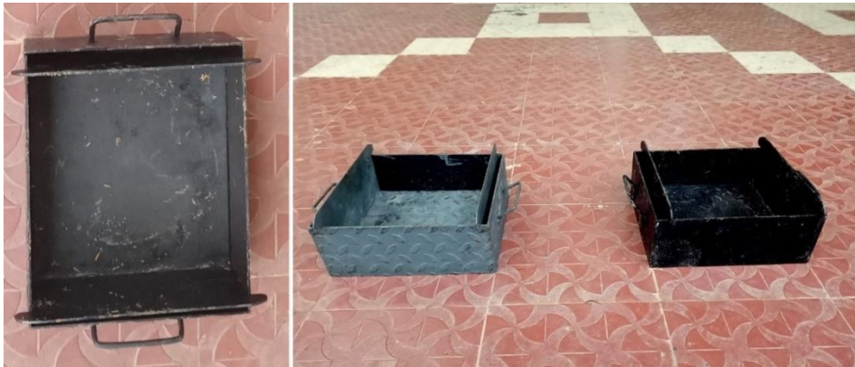
Fig.3.5: Fabricated Mould for making the thermal insulation board
