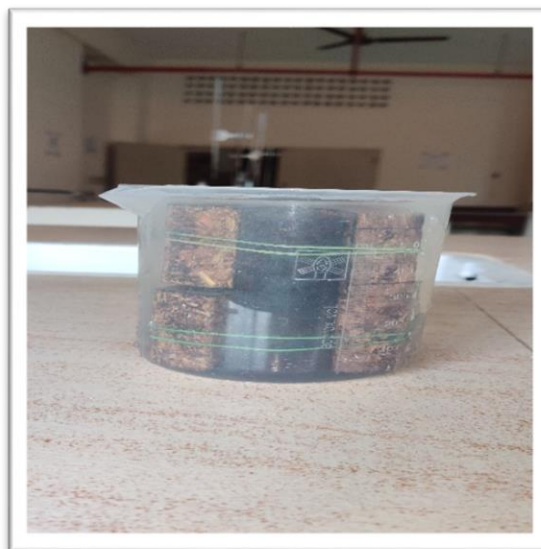
Fig.3.14: samples immersed in water for measuring thickness of swelling
