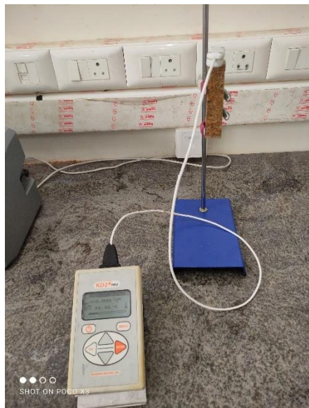
Fig. 3.17: Measurement Thermal Conductivity using KD2 pro
