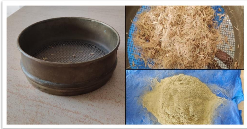
Fig. 3.3: Sieving and collection of crushed Water hyacinth petioles (particles passing through 2.36 mm IS Sieve)
