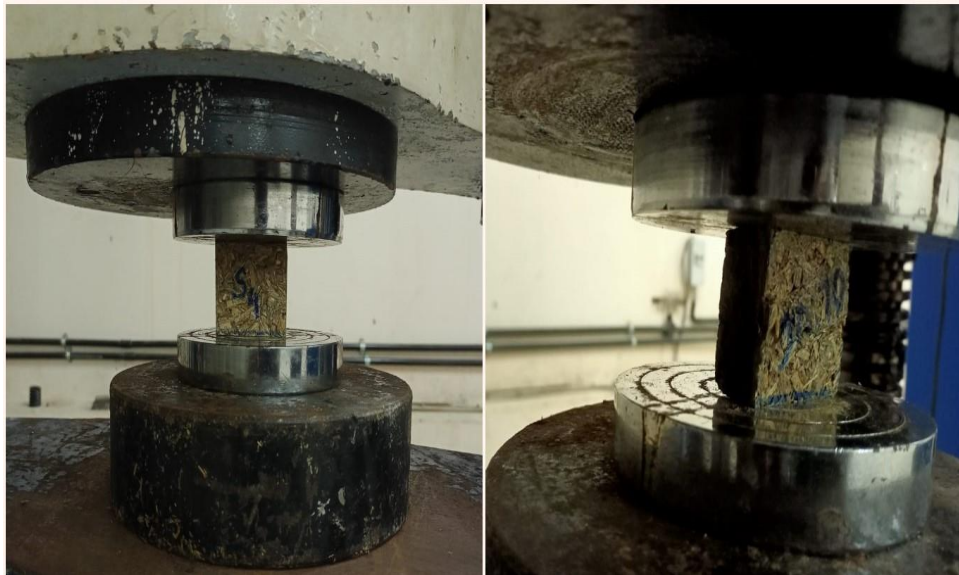
Fig. 3.16: Compressive strength measurement using UTM.
