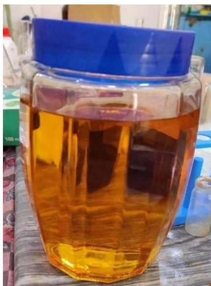
Fig. 3.11 POME obtained after transesterification
