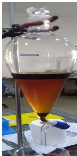
Fig. 3.8 Acid Esterification (Upper- methanol, Middle layer- oil and Lower layer -sediments)
