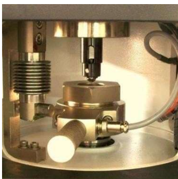
Fig. 3.19 Four ball tester [29]
