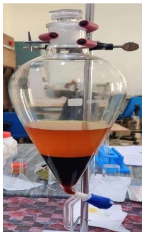
Fig. 3.9 Alkali Esterification (Top layer: POME, Bottom layer: Glycerol)
