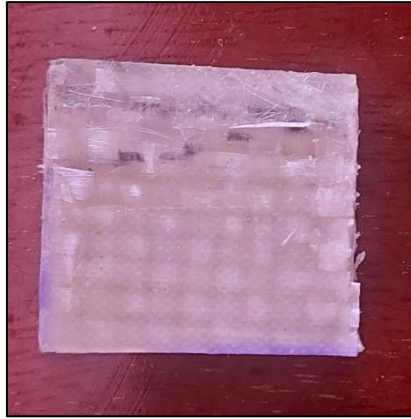
Fig.4.5 Roughness tested sample of direct sunlight cured type.
