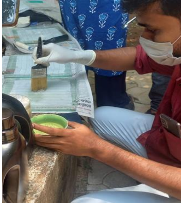
Fig.3.14 Fabrication by Hand layup.
