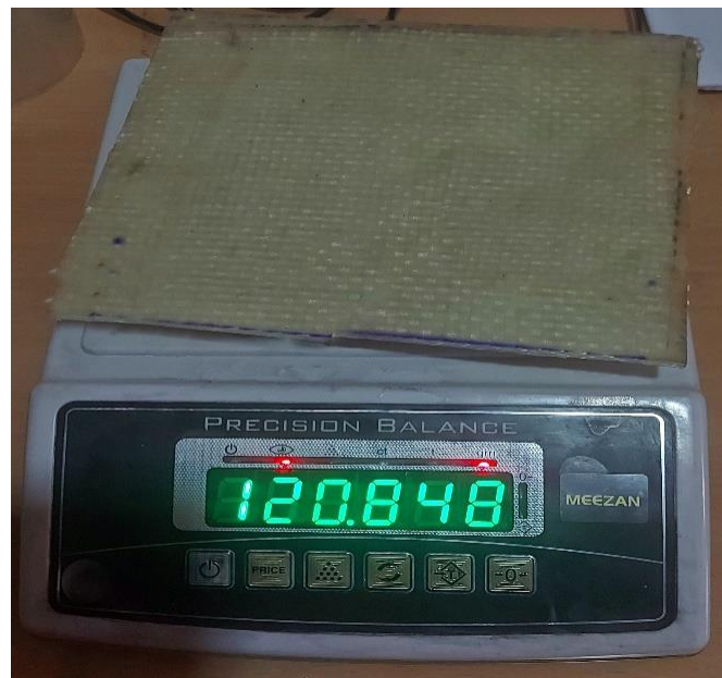
Fig.4.9 Artificial UV cured specimen weighing in precision balance.
