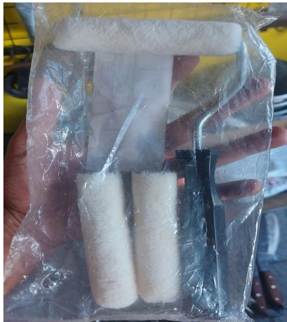
Fig.3.9 Roller brush used for pressurizing.
