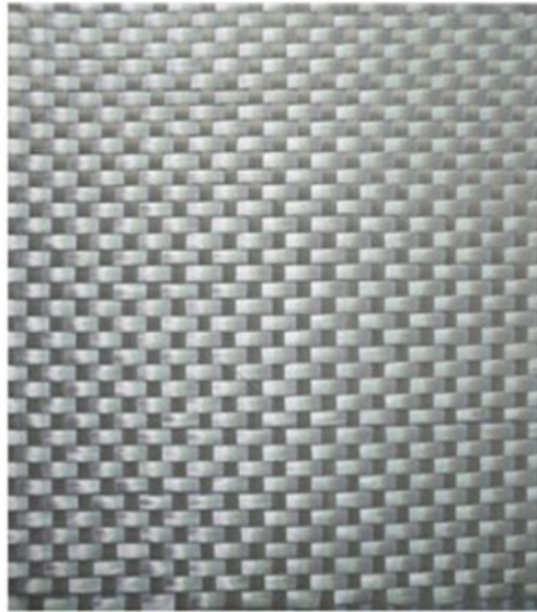
Fig.3.3 Glass fibre used as reinforcement.
