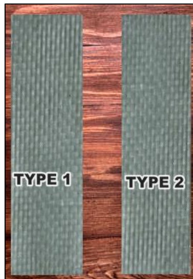
Fig.4.7 Specimens of each type submitted for tensile strength test.
