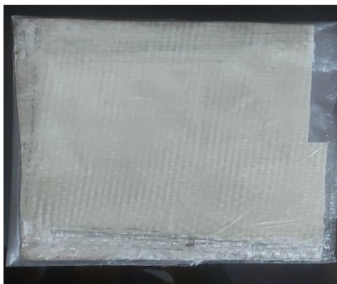
Fig.4.2 UV A type lamp cured specimen for testing.
