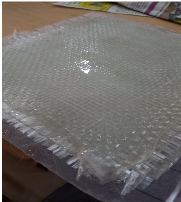
Fig.3.13 Glass fibre placing.
