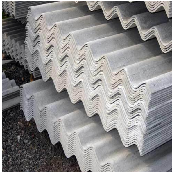
Fig 1.16: Asbestos cement roofing sheets
