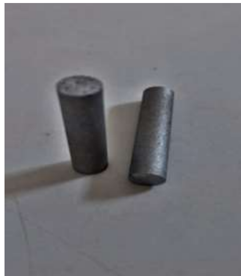
Fig 5.2 Specimen (ASTM G99 standard)
