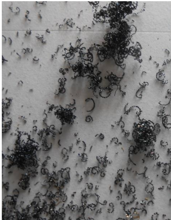
Fig No. 8.2 Form B-Helical broken chips of length ranges from 0.5 - 2 inch.
