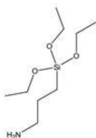
Fig. 3.7. Chemical structure of 3-APTES
