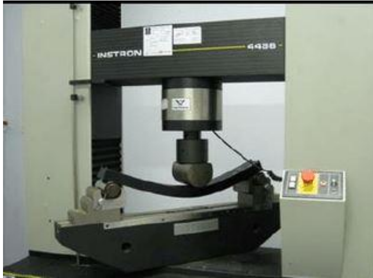
Fig. 4.9. Experimental set up for 3-point bending test
