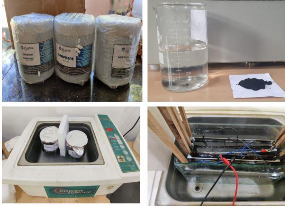
Fig. 3.11. Experimental setup for the EPD process
