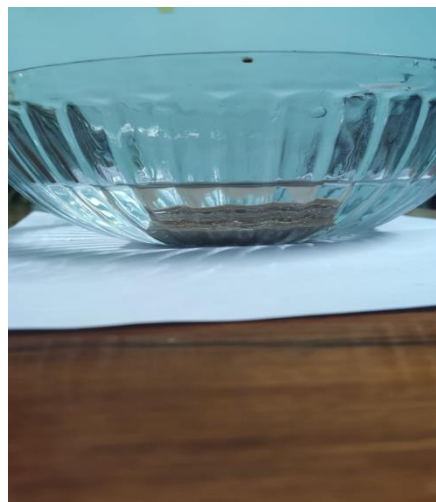
Fig.4.12 HFRP sample kept in distilled water
