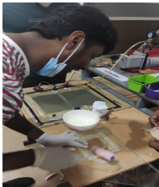
Fig.3.12 Hand layup Procedure (Space lab, TKMCE).
