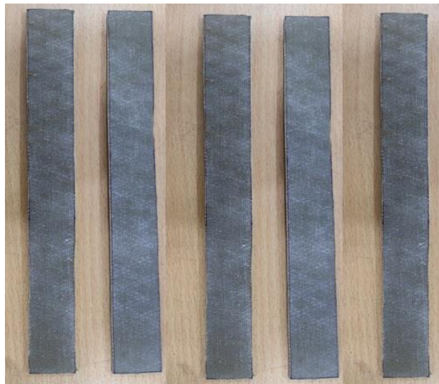
Fig 4.4 Tensile test specimen (ASTM D3039)
