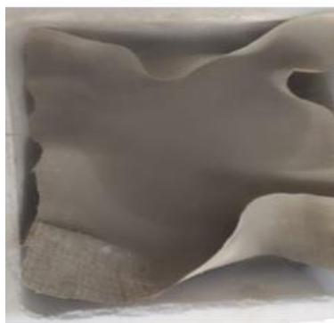
Fig.3.18 Hemp woven cloth in cryo-bath
