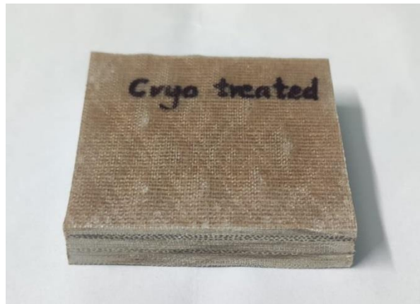
Fig.3.13 HFRP fabricated by Hand layup method
