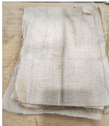
Fig.3.3 Unidirectional Hemp Fiber mat Twill type used as reinforcement.
