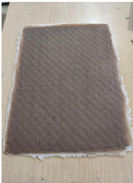
Fig.4.1 Fabricated composite by VARTM
