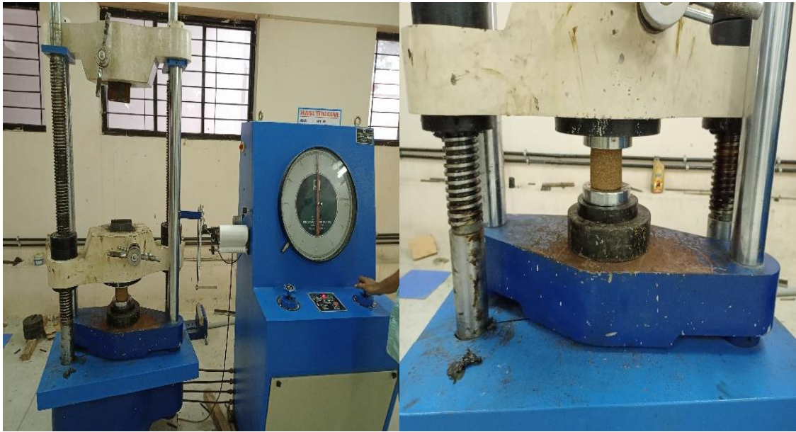
Fig 3.26 Compressive strength test of briquette sample in UTM
