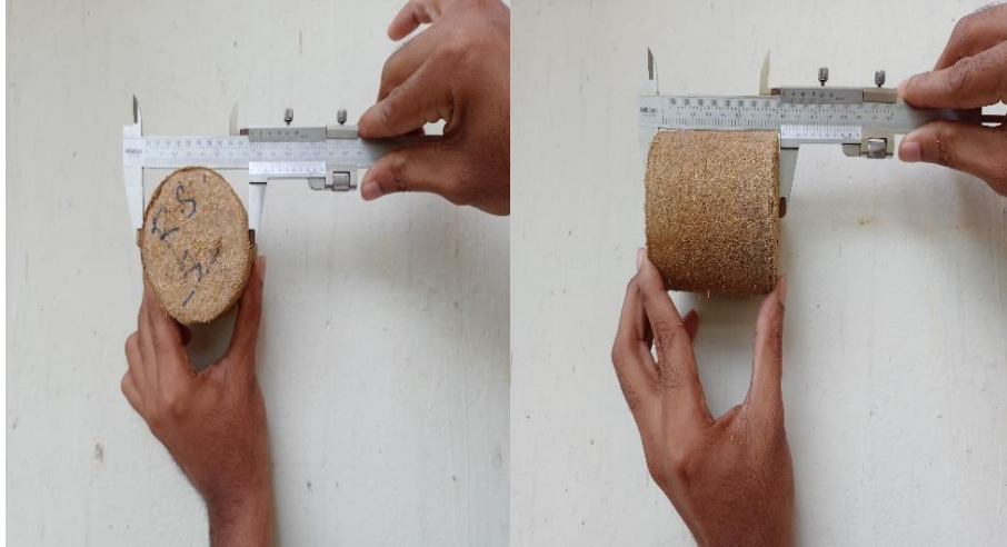
Fig 3.21 Measuring dimensions using vernier callipers
