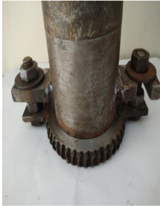
Fig 3.16 Locking arrangement in mold
