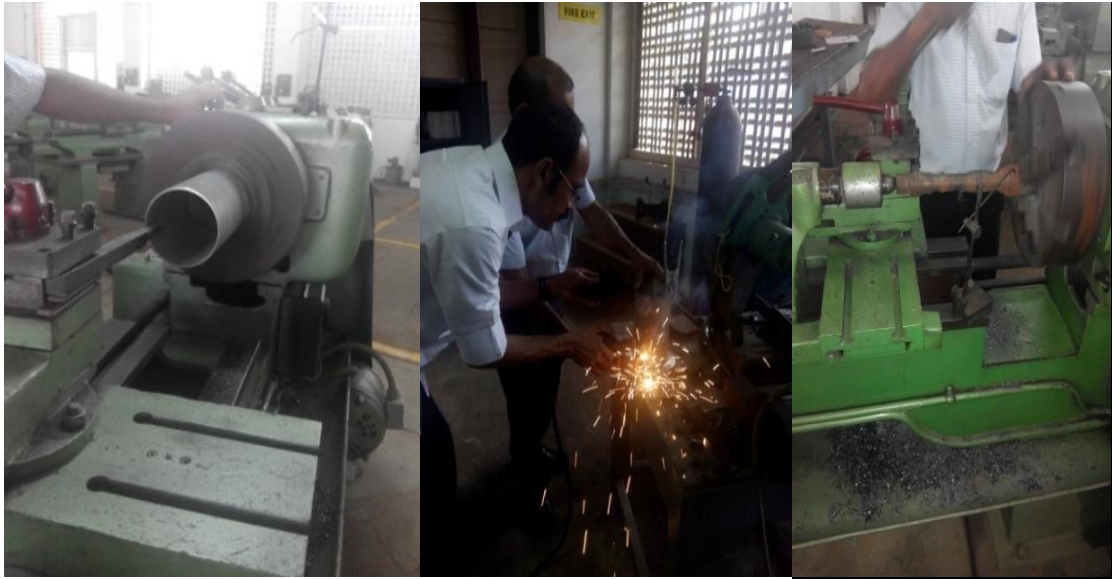
Fig. 3.14 Mould fabrication processes -boring welding and shaping
