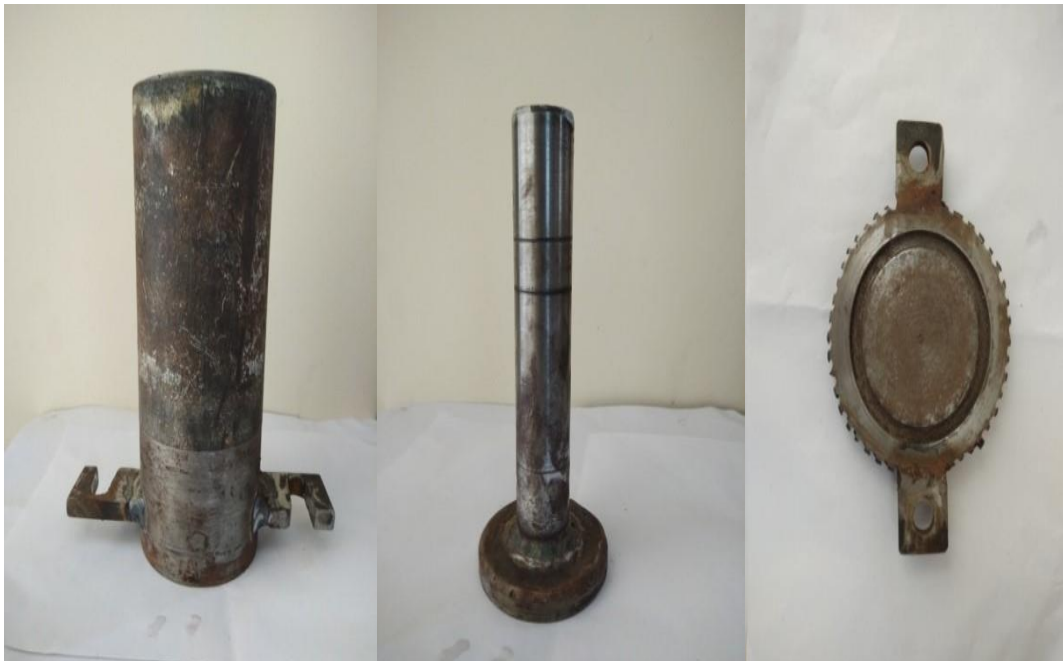
Fig. 3.15 Mould components- cylindrical die, piston and a base plate
