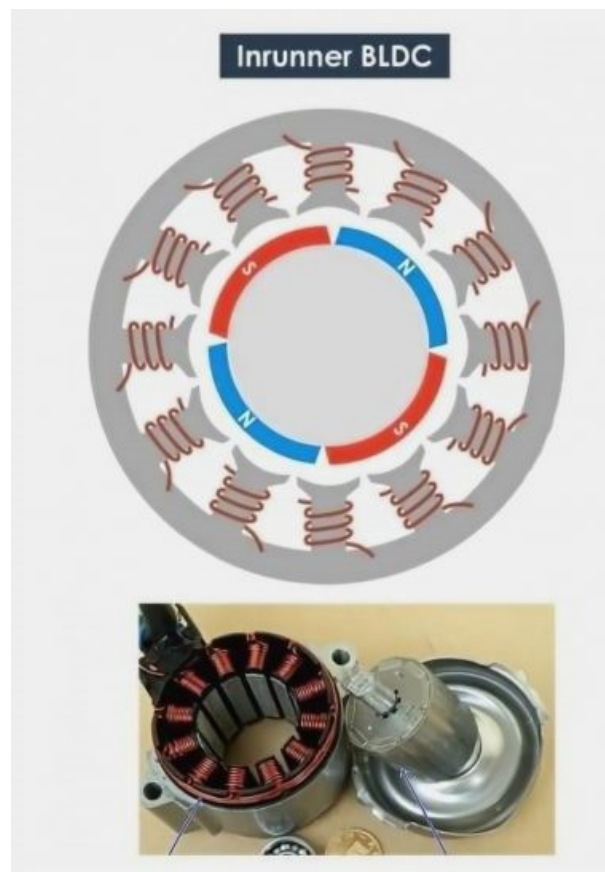
Figure 3.2: Inner rotor BLDC motor
