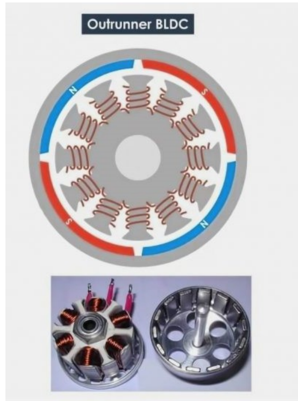
Figure 3.3: Outer rotor BLDC motor
