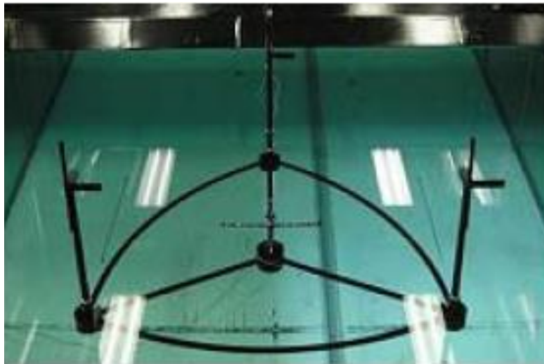
Fig. 2.15 Model of semi-submersible platform for three wind turbine towers (Ishihara et al. 2007)
