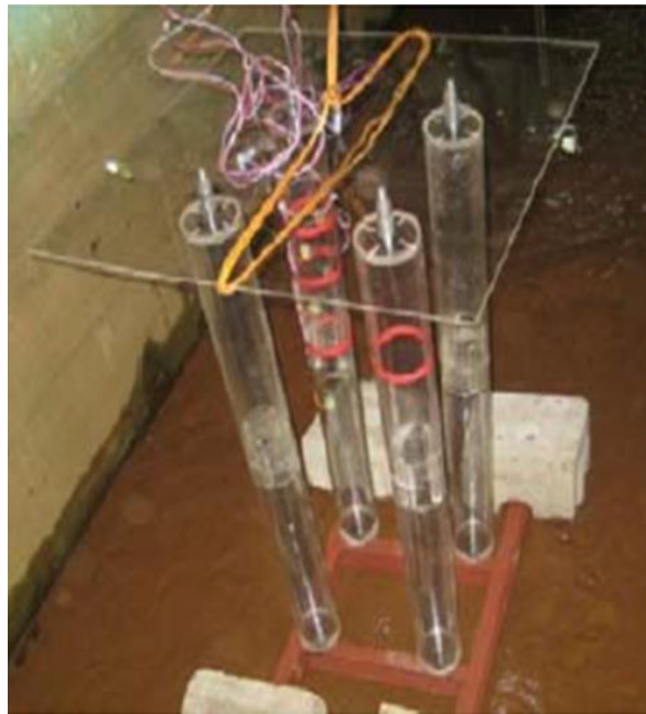
Fig.2.12 Model of three-leg articulated tower (Nagamani and Ganapathy 2000)
