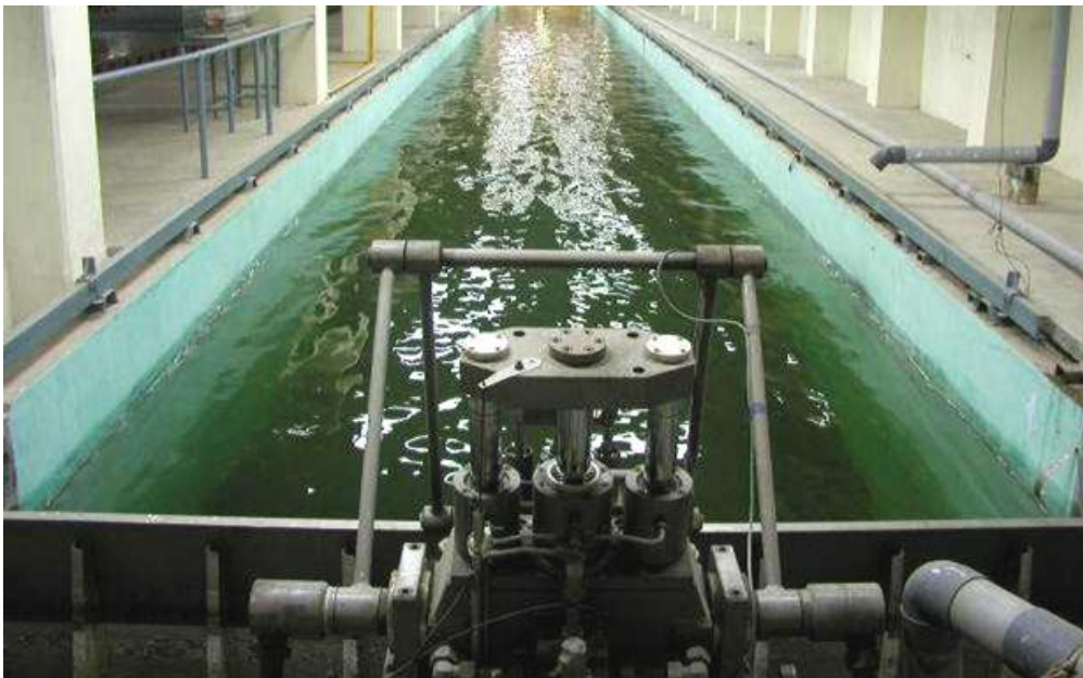
Fig.4.3 Wave flume with wave maker
