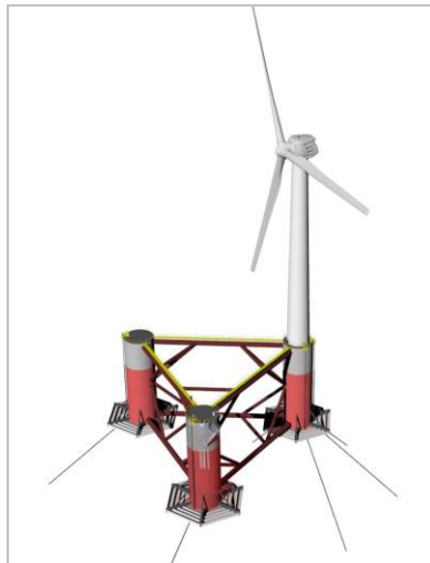
Fig.2.5 WindFloat Concept (Roddier et al. , 2009)
