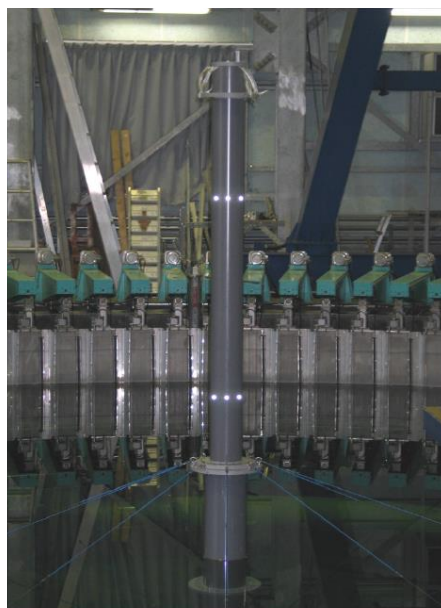
Fig.2.16 Scale model of SPAR-type platform at NMRI (Utsunomiya et al. 2009)
