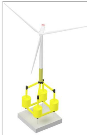
Fig.2.10 TLP designed by GICON (Kausche et al. 2018)
