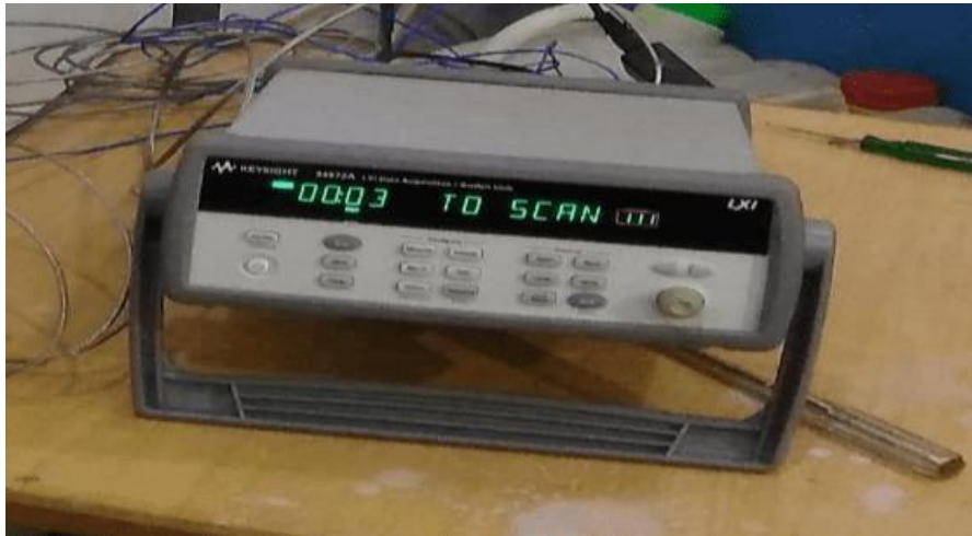
Fig 4.10 Data acquisition system
