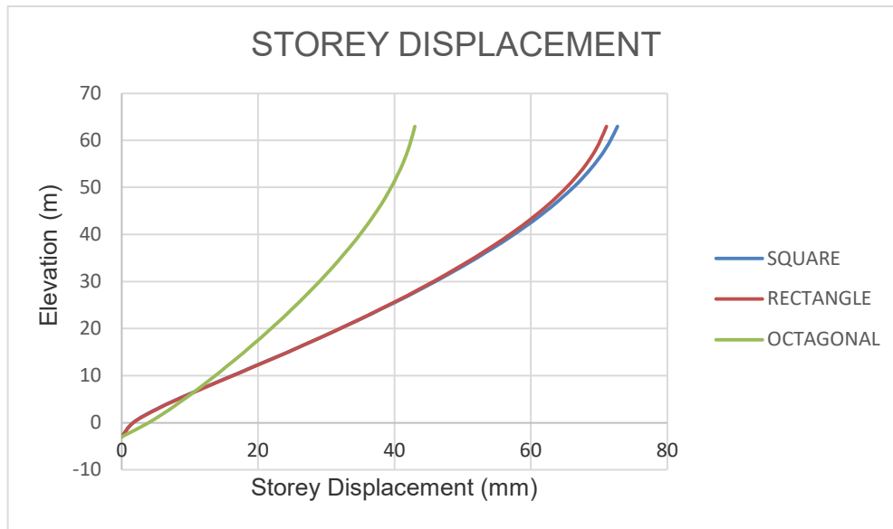
Figure.9.23 Storey Displacement for Zone V
