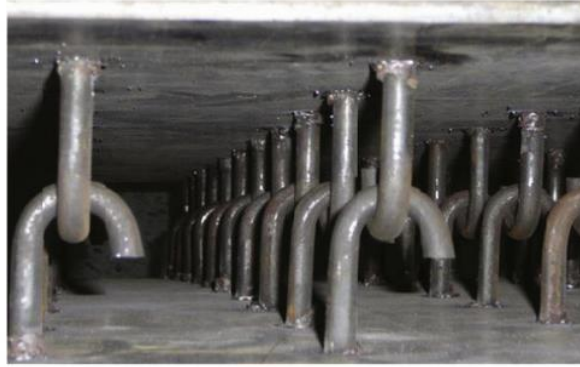
Figure 2.3 J-hook connectors (Liew et al., 2017)
