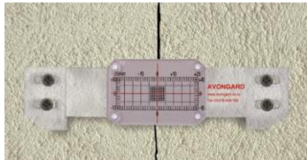
Figure 1.7: Crack width ruler for measuring crack width
