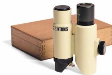
Figure 1.6: Crack width microscope for measuring crack width
