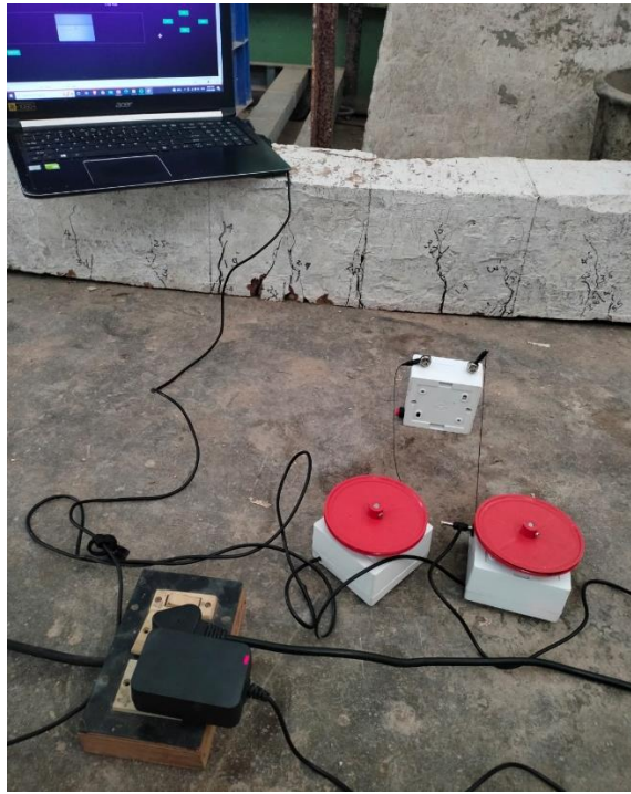
Figure 6.6: Crack Analysis using proposed equipment
