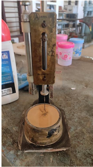
Fig. 5.16: Setting time test on AAP of 100% slag with 0.8M phosphoric acid and red gypsum at 2.5% of binder content
