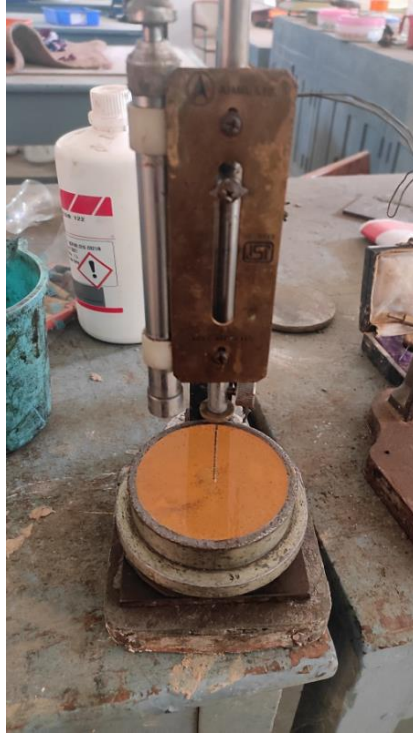
Fig. 5.19: Setting time test on AAP with 0.5M phosphoric acid and red gypsum at 2.5%
