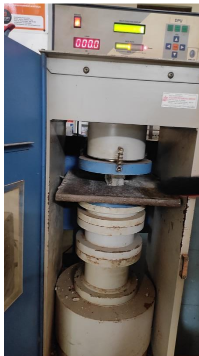
Fig. 4.6 Digital compression testing machine for compressive strength test on 40 \times 40 \times 40 \text{ mm}^3 cube specimens
