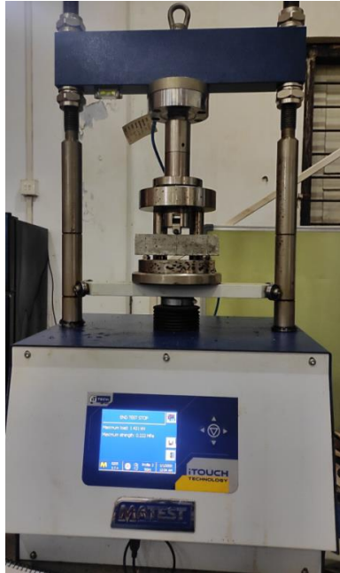
Fig. 4.5 Multi frame testing apparatus for flexural strength test on 40 \times 40 \times 160 \text{ mm}^3 AAM Prism specimens
