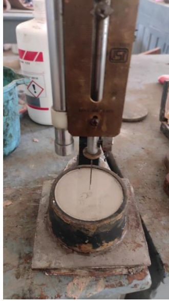
Fig. 5.17: Setting time test on AAP with 0.8M phosphoric acid as admixture
