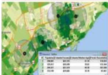
Geographic overlay/aggregation is supported and allows attribute assignment between layers based on percentage overlap for estimating demographics of territories, buffers, areas of influence, and more
