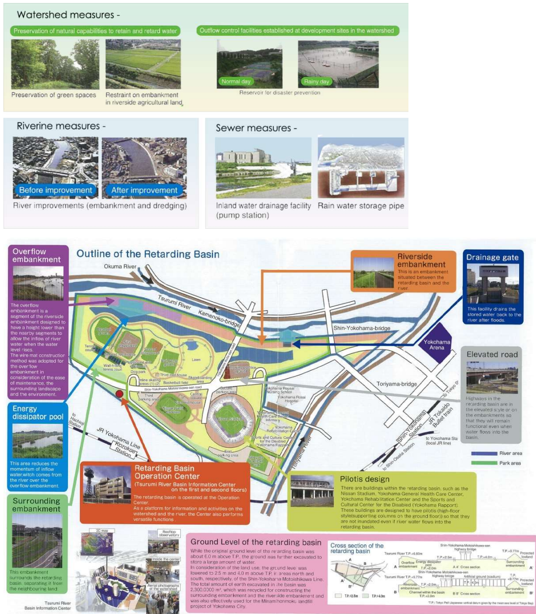
Figure 23 - Comprehensive Flood control measures.
