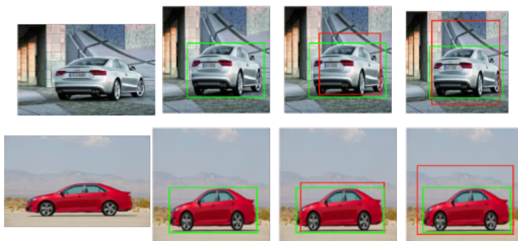
Figure 4.4: Localization results on Stanford Cars-196. Figure shows input image, Ground Truth, Localized result from proposed method and Localized result from OLM method respectively
