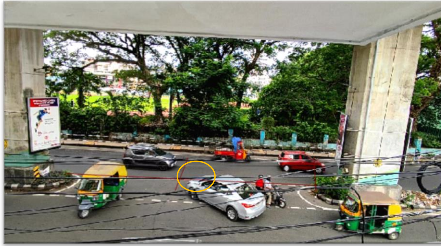
Figure 4.17. Time t_0 when the Front Bumper of a Vehicle Crosses Reference Line
