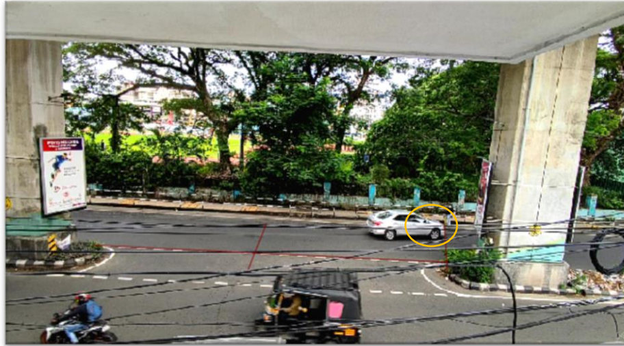
Figure 4.23. Time t_6 when the Front Bumper of a Vehicle Crosses Reference Line
