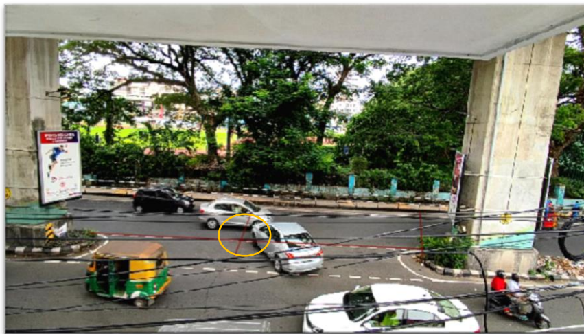
Figure 4.18. Time t_1 when Initial Portion of Vehicle Crosses Reference Line
