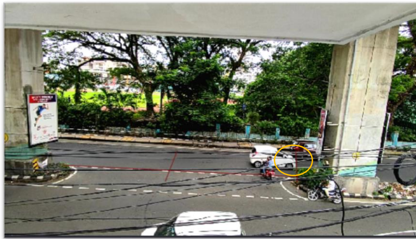
Figure 4.15. Time t_2 when the Front Bumper of a Vehicle Crosses Reference Line
