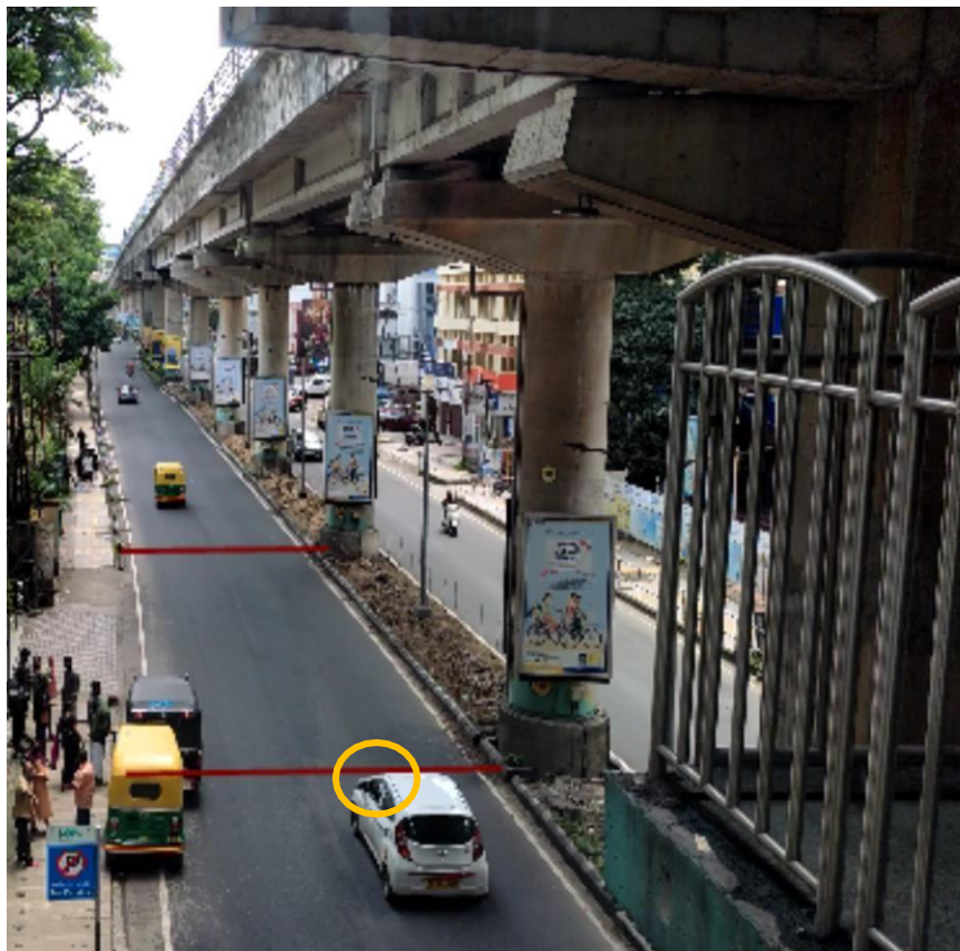
Figure 4.7. Time t_3 when Vehicle Enters the Trap Length
