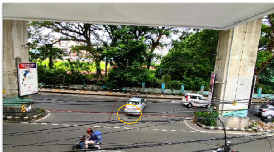
Figure 4.22. Time t_5 when the Back Bumper of a Vehicle Crosses Reference Line
