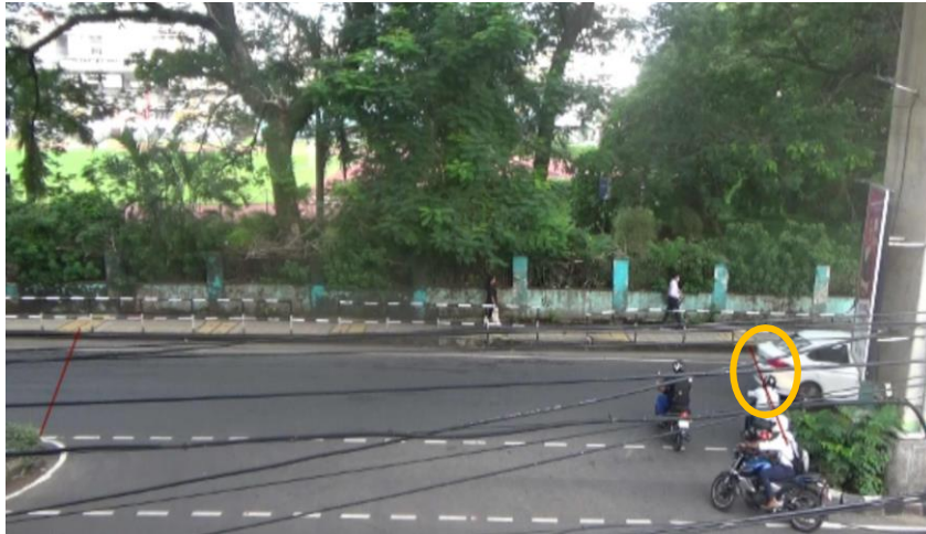
Figure 4.6. Time t_2 when Back Bumper of Vehicle Leaves the Median Opening
