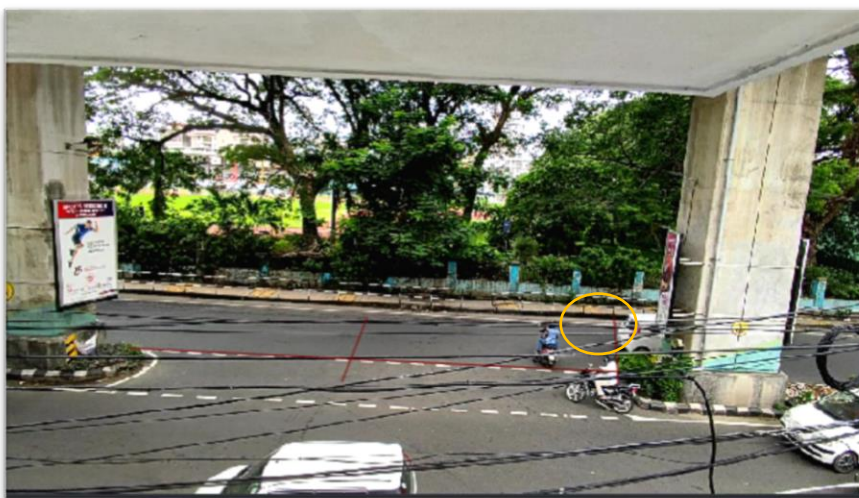
Figure 4.16. Time t_3 when the Back Bumper of a Vehicle Crosses Reference Line
