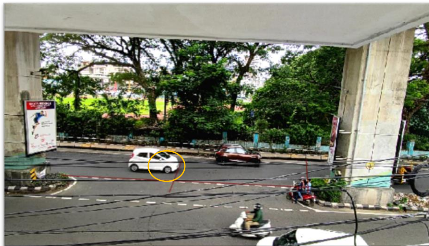
Figure 4.13. Time t_0 when the Front Bumper of a Vehicle Crosses Reference Line
