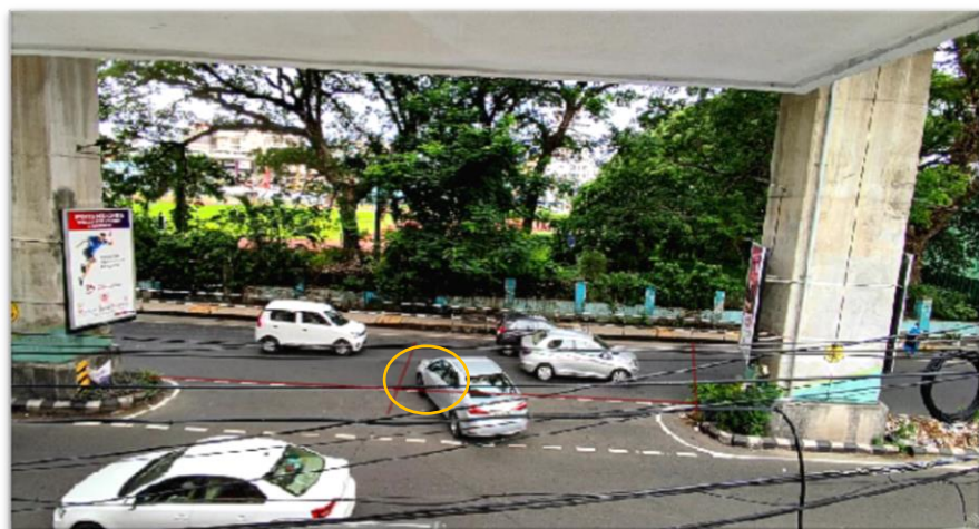
Figure 4.19. Time t_2 when Initial Portion of Vehicle Crosses Reference Line after Stoppage
