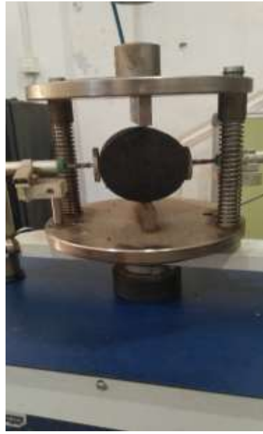
Fig. 3.12 ITS testing machine
