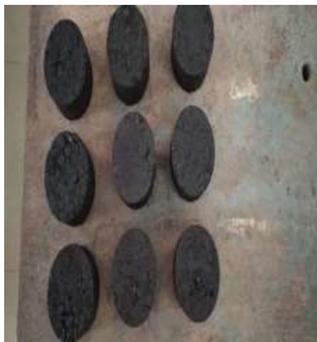
Fig. 3.9 Specimens for ITS
