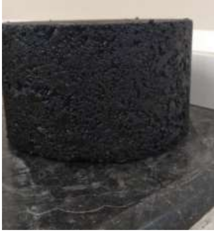
Fig. 3.13 Specimen for rut test
