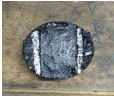
Fig. 3.16 Specimen after rut test
