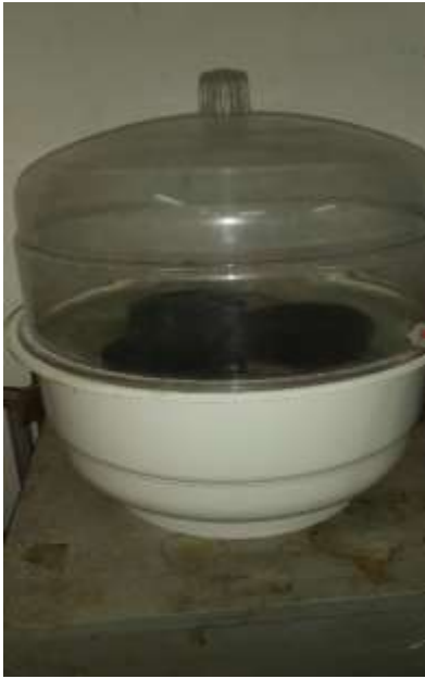
Fig. 3.11 Specimens in vacuum container
