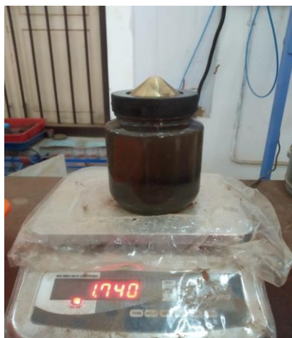
Figure 3.14 Specific gravity test performed using pycnometer
