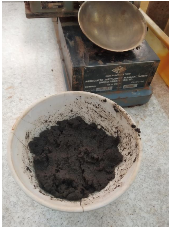
Figure 3. 16 Soil sample collected from Kainakary about to be tested in Casagrande apparatus.
