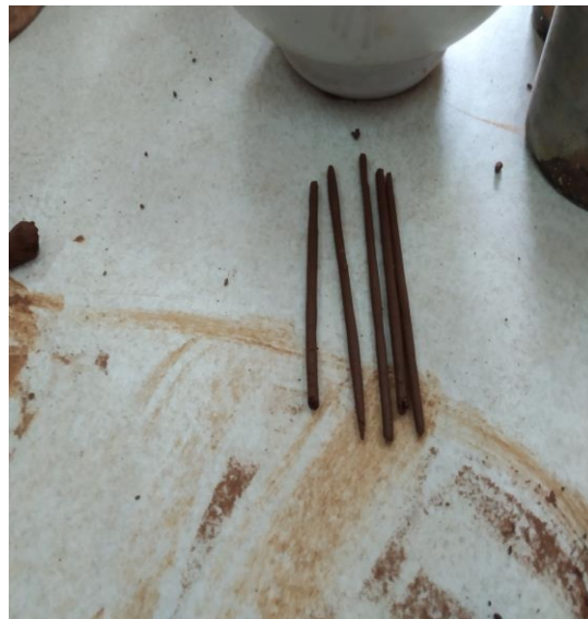
Figure 3. 18 Soil rolled down to threads of 3 mm diameter
