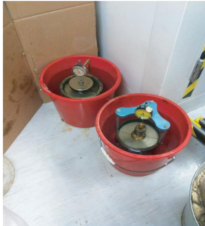
Figure 2. 1 Experiment to test the volume change of soaked soil specimens with surcharges (Source: Wang et al., 2014)
