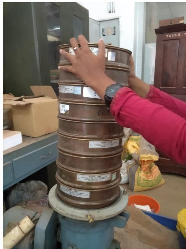
Figure 3. 15 Sieve analysis test performed using various IS sieves in sieve shaker
