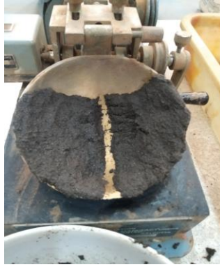
Figure 3. 17 Liquid limit test performed in Casagrande apparatus for soil sample collected from Kainakary
