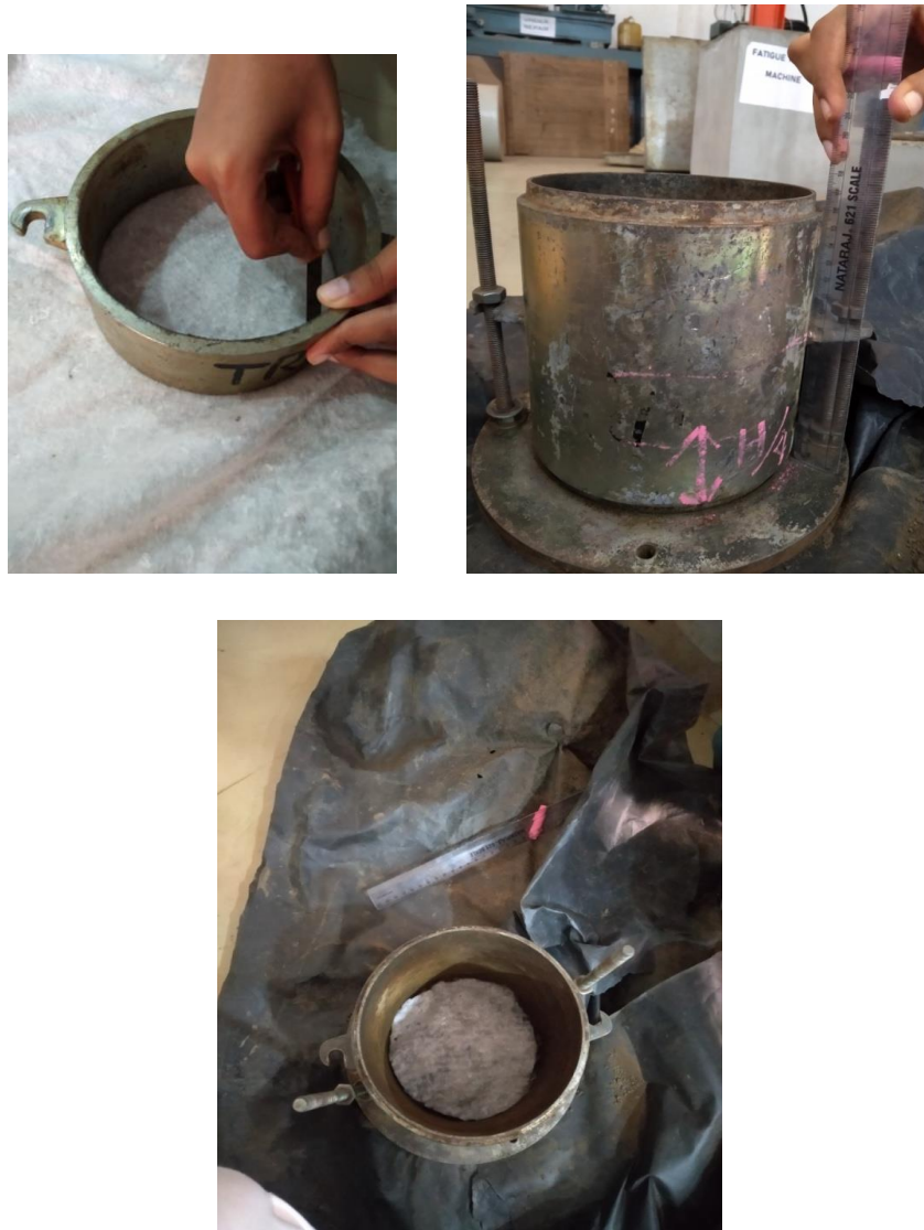
Figure 3. 28 CBR mould with geotextile being kept in position
