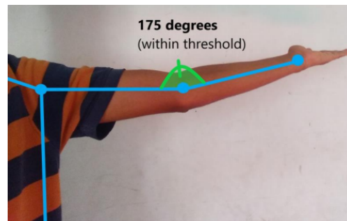
Figure 3.7: User's Hand Pose Of 175 Degrees Is Within The Threshold Of + or -5 Degrees
