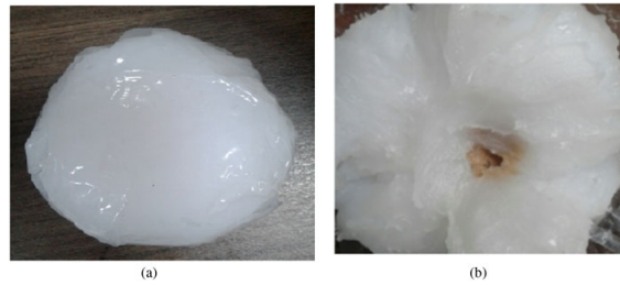
Figure 2.3: (a) Breast phantom (b) Tumor made of wheat flour at center of breast phantom [10]
