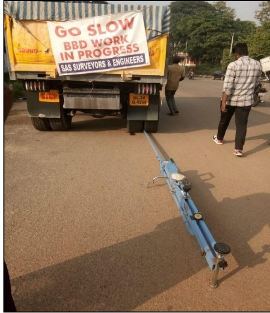
Fig. 4.2 Conducting BBD test on pavement surface
