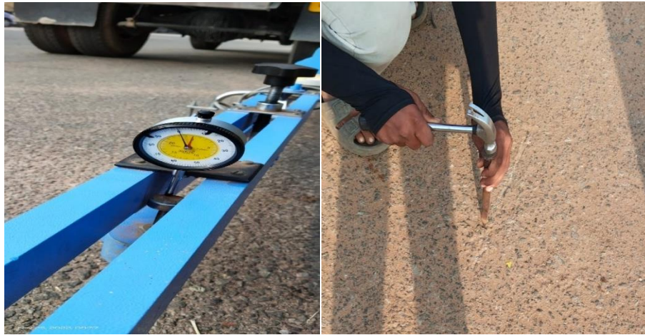
Fig. 3.2 (a) Setting dial gauge to BBD (b) Testing pavement temperature
