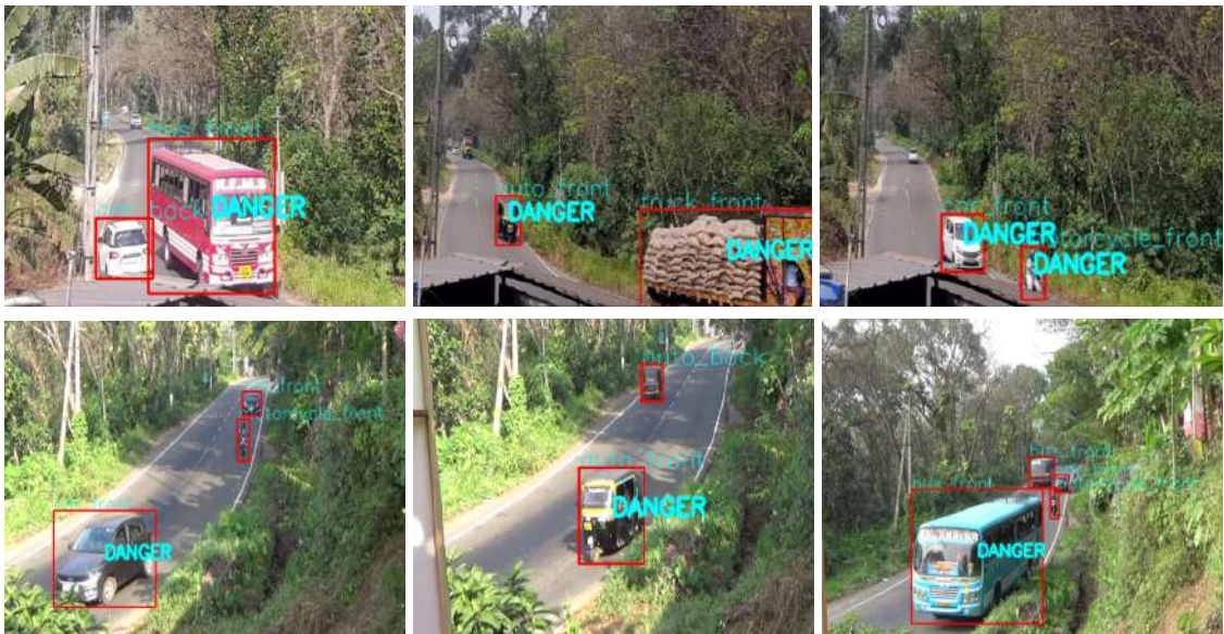
Figure 8.28 Detecting the Dangerous Vehicle Coming into the Curve
