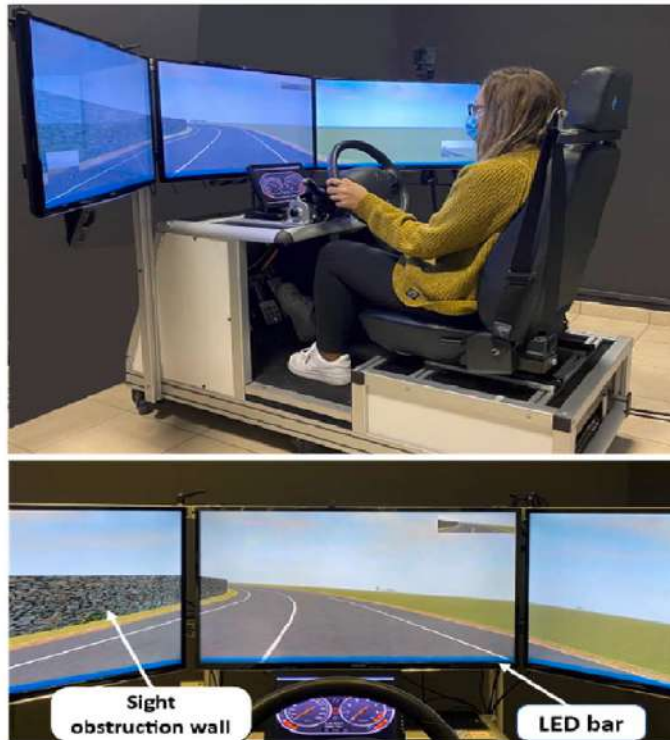
Figure 2.4 The Virtual Scenario Setup for the Experiment (Source: Hazoor et al., 2022)
