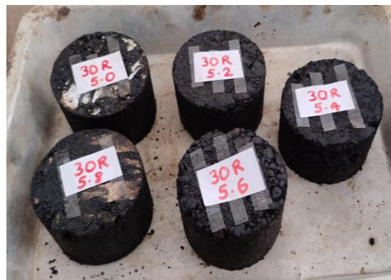
Figure 4.11 Samples with 30% RAP materials
