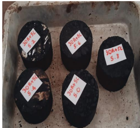
Figure 4. 15 Samples with 30% RAP+ 5%Castor oil
