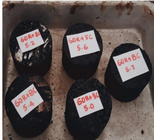
Figure 4. 17 Samples with 60% RAP+ 8%Castor oil
