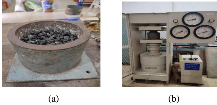
Figure 3.10 Aggregate Crushing Strength Test (a) Mould with Aggregates, (b) Crushing Strngth Testing Machine
