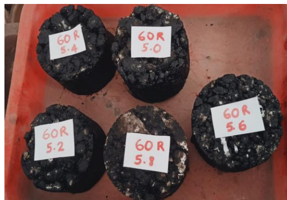
Figure 4.13 Samples with 60% RAP materials
