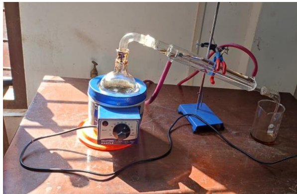
Figure 3.6: Primary Distillation Unit
