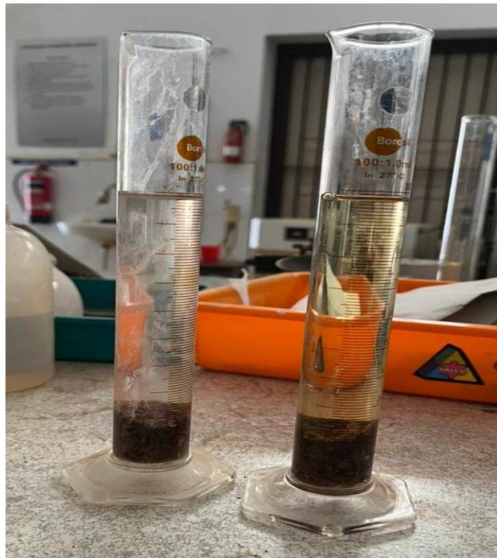
Figure 3.8- Swelling Test on Soil
