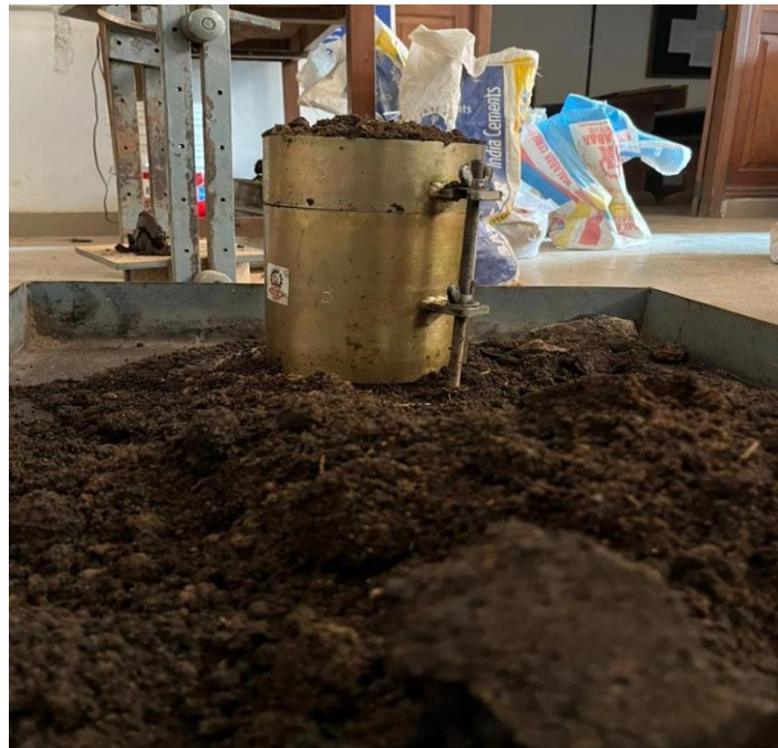
Figure 3.6- Preparation of CBR Specimens
