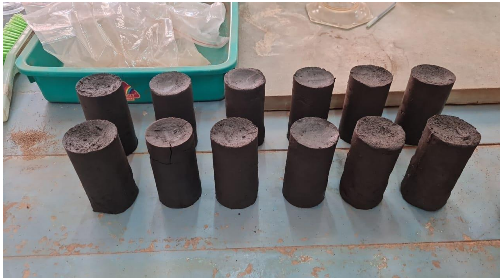
Figure 3.7- Casted Specimens for Compression Test
