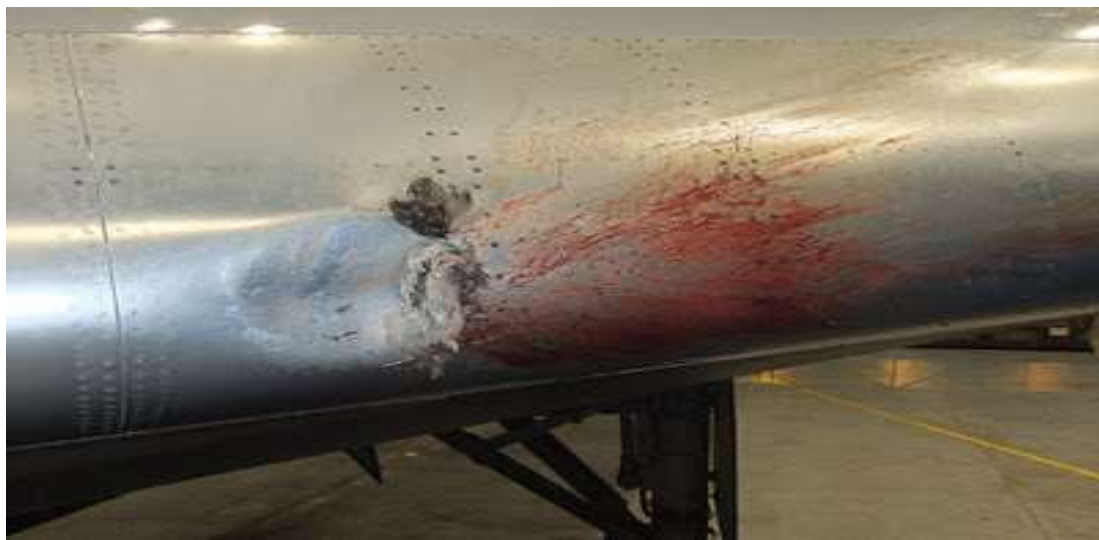
Fig 1.1 Aircraft leading edge struck by bird
