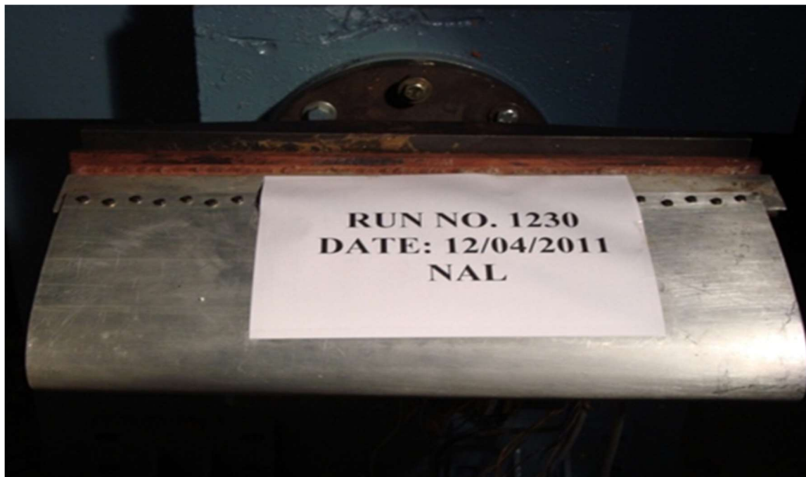
Fig 4.4 The profile of aluminium alloy (AA 2024-T3) wing leading edge before soft body impact experimental test
