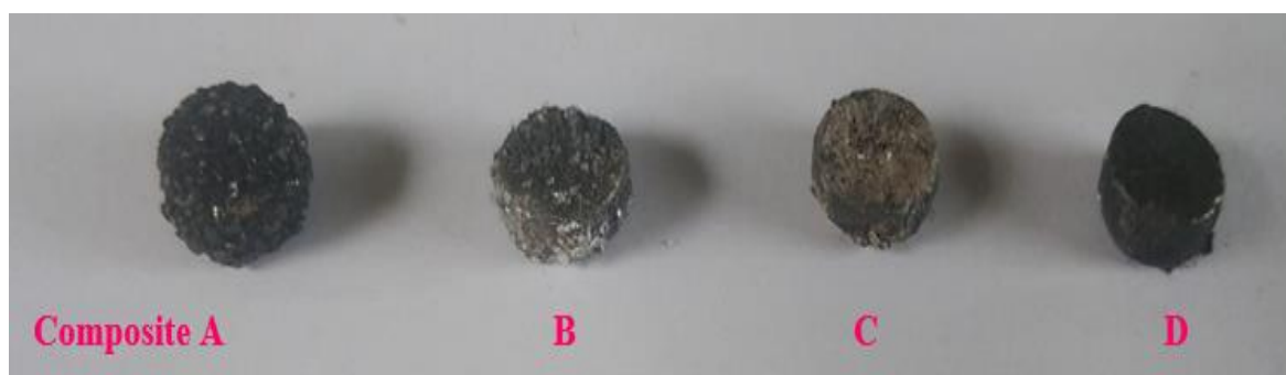
Fig. 7.3: Photograph of composite activated carbon samples prepared for the study
