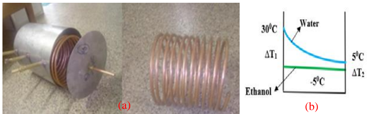
Fig. 6.2: (a) Photograph of the evaporator assembly and (b) Log Mean Temperature difference of the working fluid in evaporator
