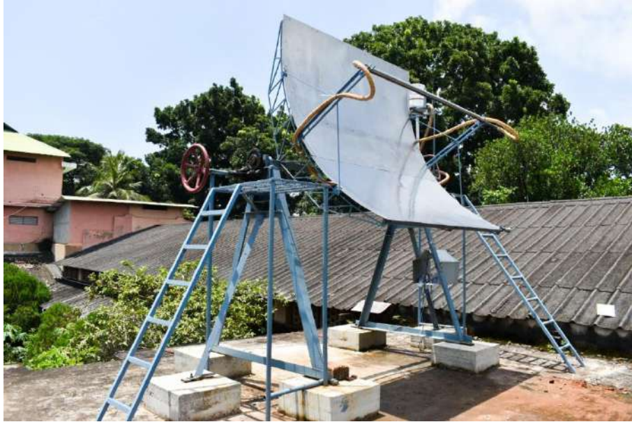
Fig. 5.23: Constructed PTC experimental setup
