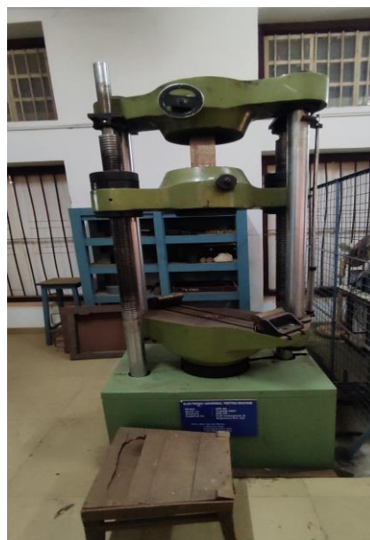
Fig 3.4 Tensile testing setup
