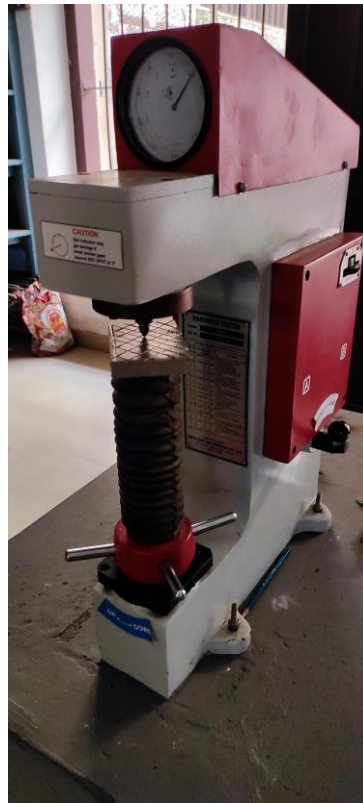
Fig 3.5 Rockwell hardnes setup
