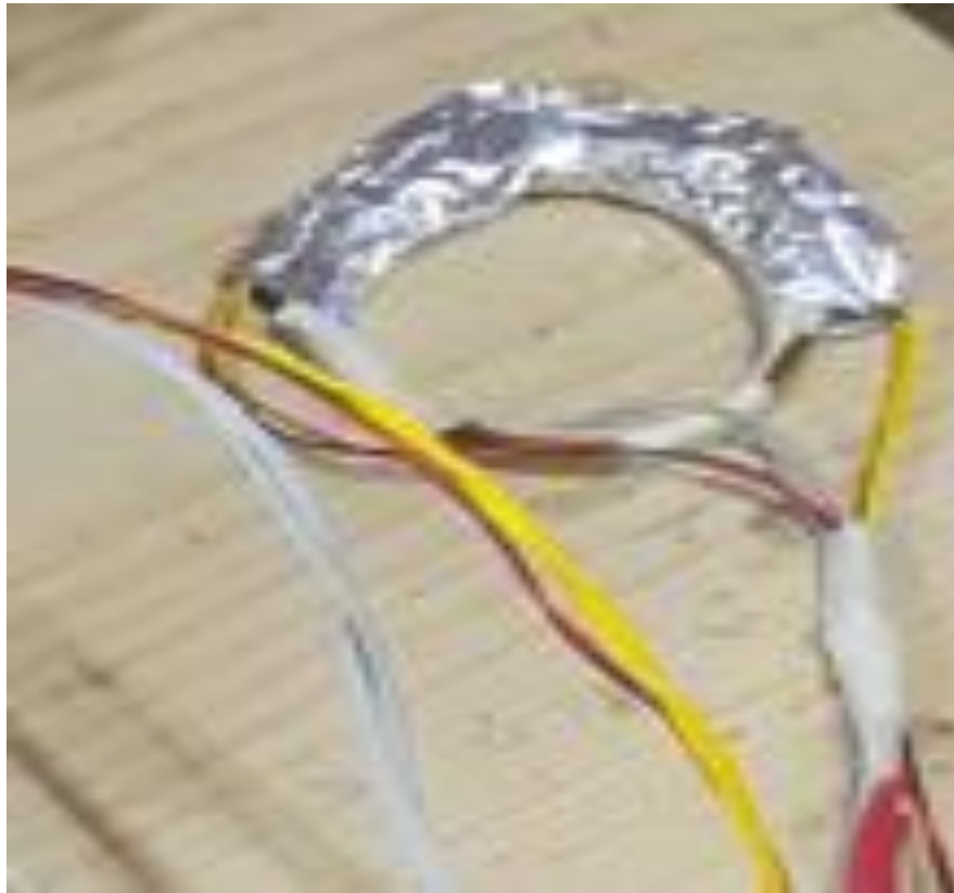
Fig 5.4: HTS attached with PT100 sensor and the specimen is insulated
