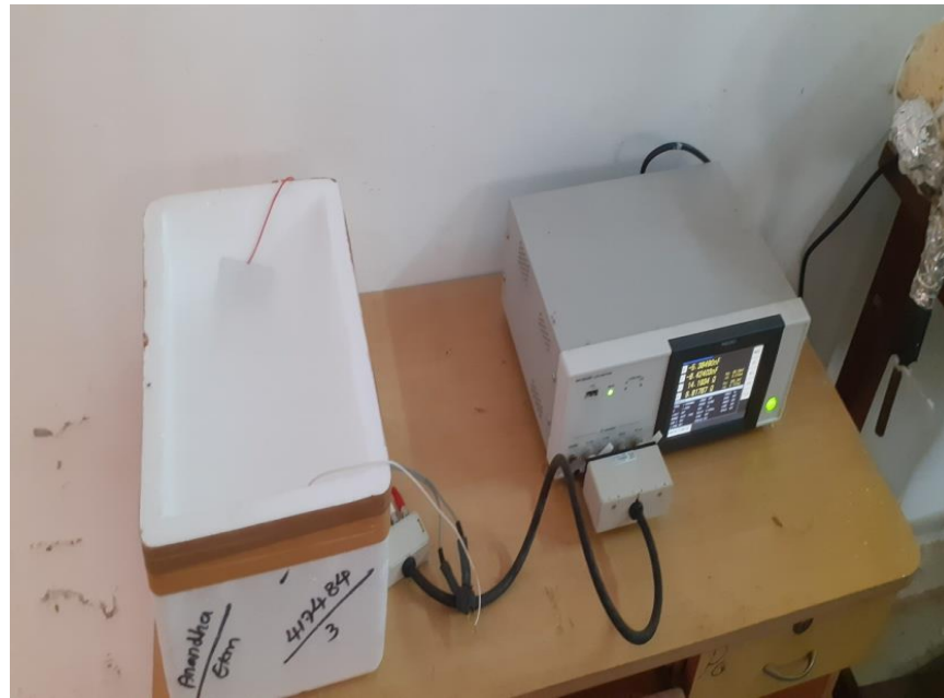
Fig 4.3: Setup for measuring resistance at LN2 temperature
