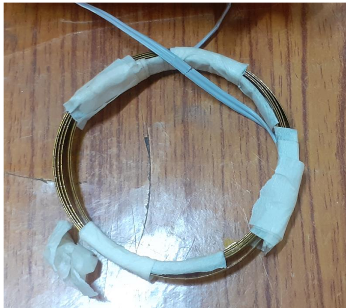
Fig 5.3: HTS attached with lead wires
