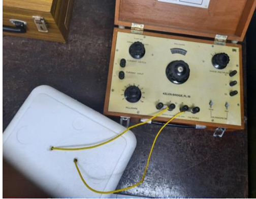
Fig 4.1: connection of specimen at LN2 temperature to Kelvin double bridge
