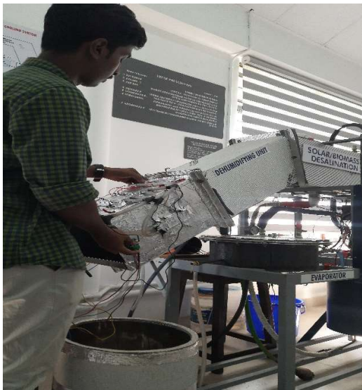
Fig. 5.18 Integrating TED with the ADS system
