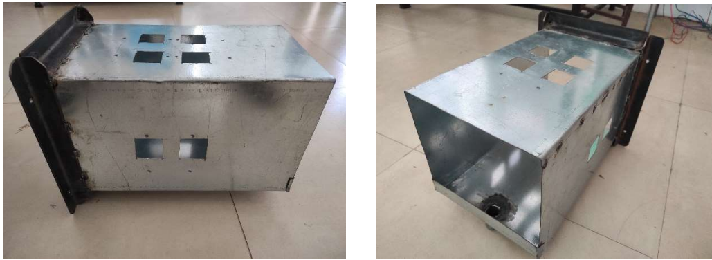
Fig. 5.8 Developed duct system using GI sheet
