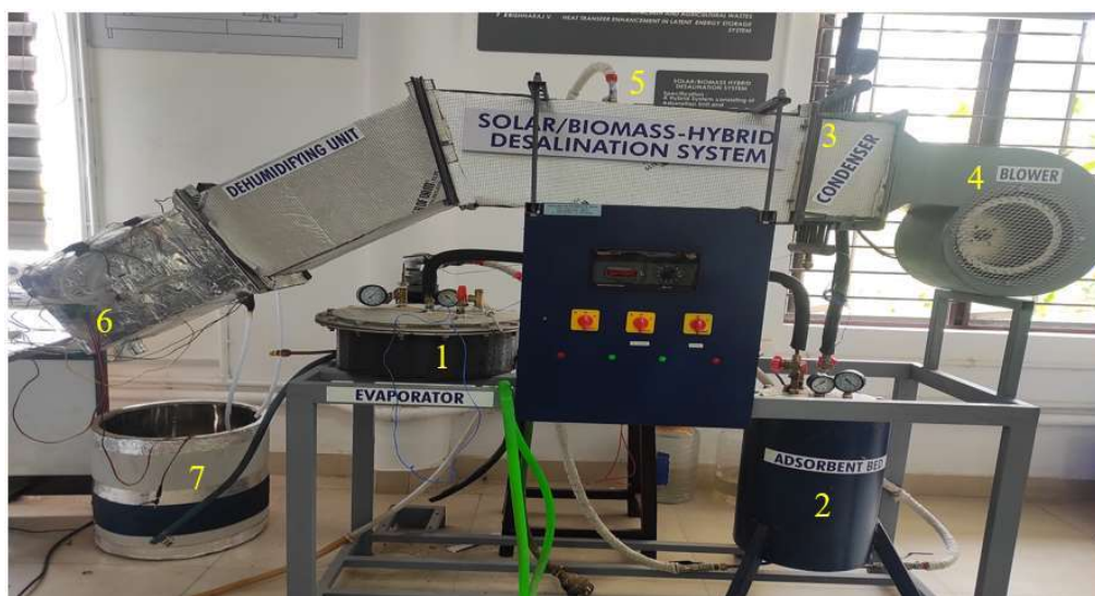
Fig. 5.16 Experimental setup of TED integrated adsorption desalination system
