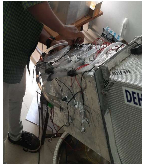
Fig. 5.18 Integrating TED with the ADS system
