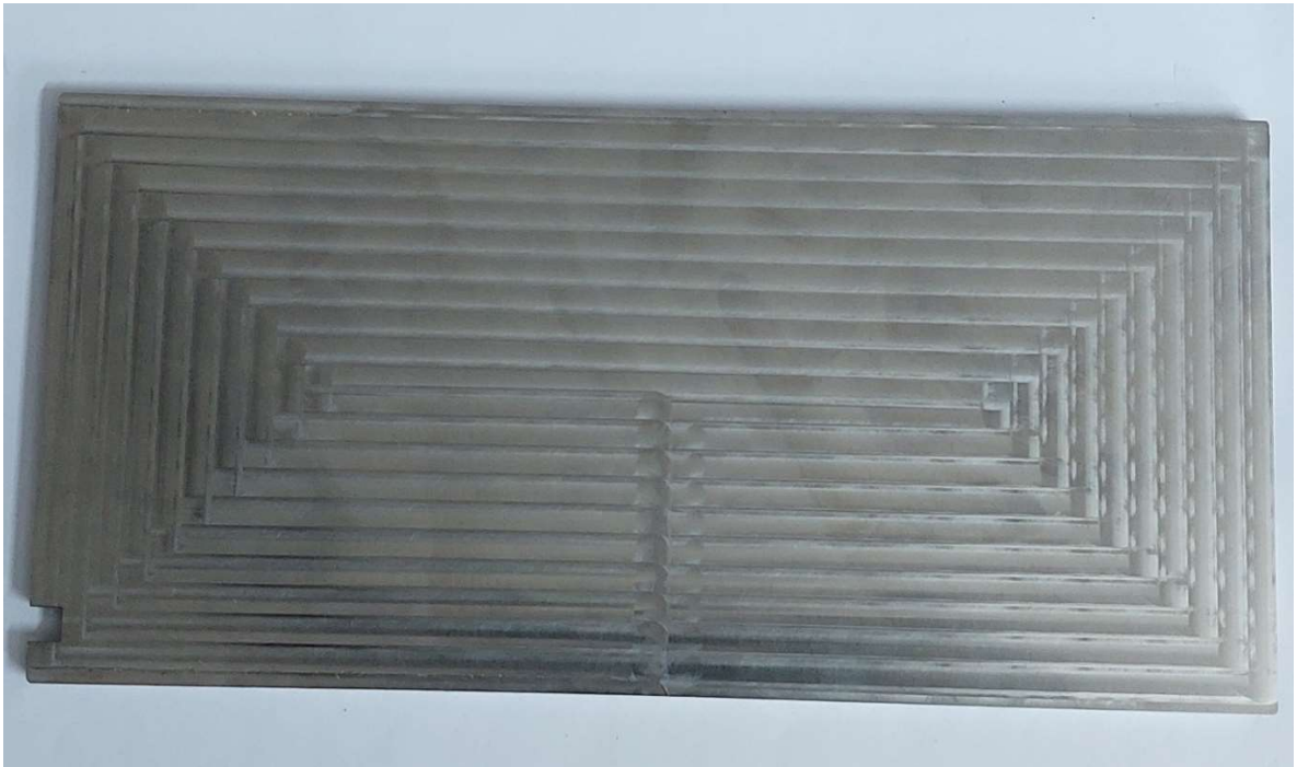
Fig 3.1 200*100*8mm maraging steel plate
