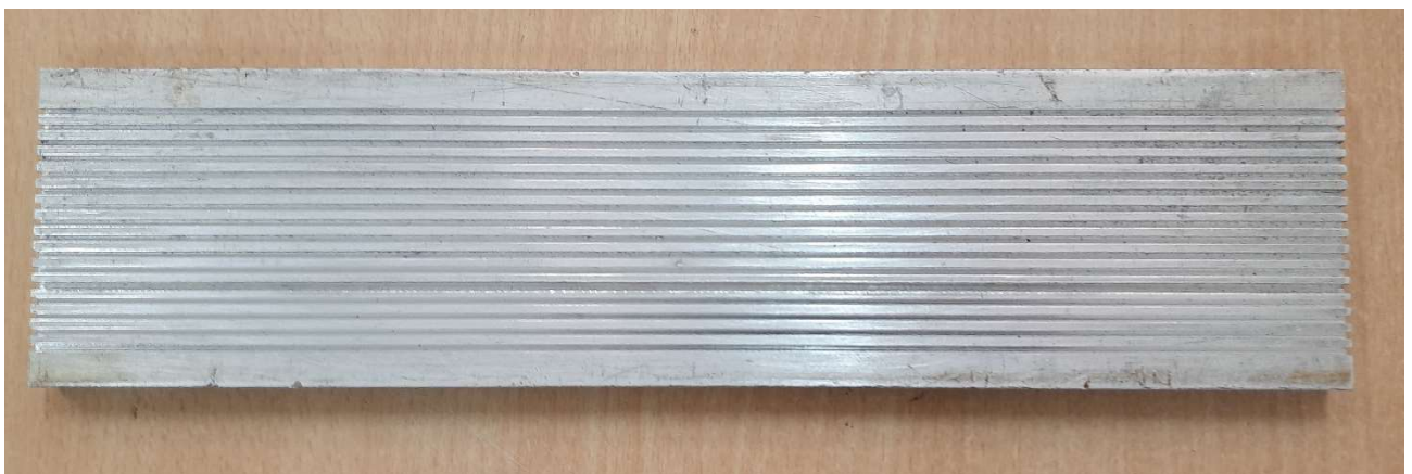
Fig: 4.10. Machined aluminium base plate for 2mm channel width
