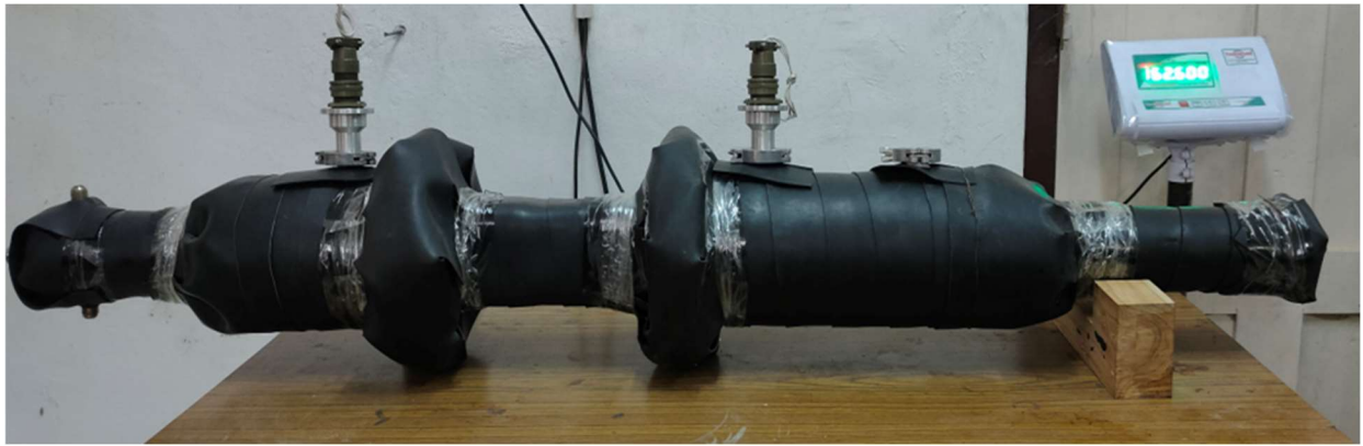
Fig: 4.20. Assembled section after applying Nitrile Rubber
