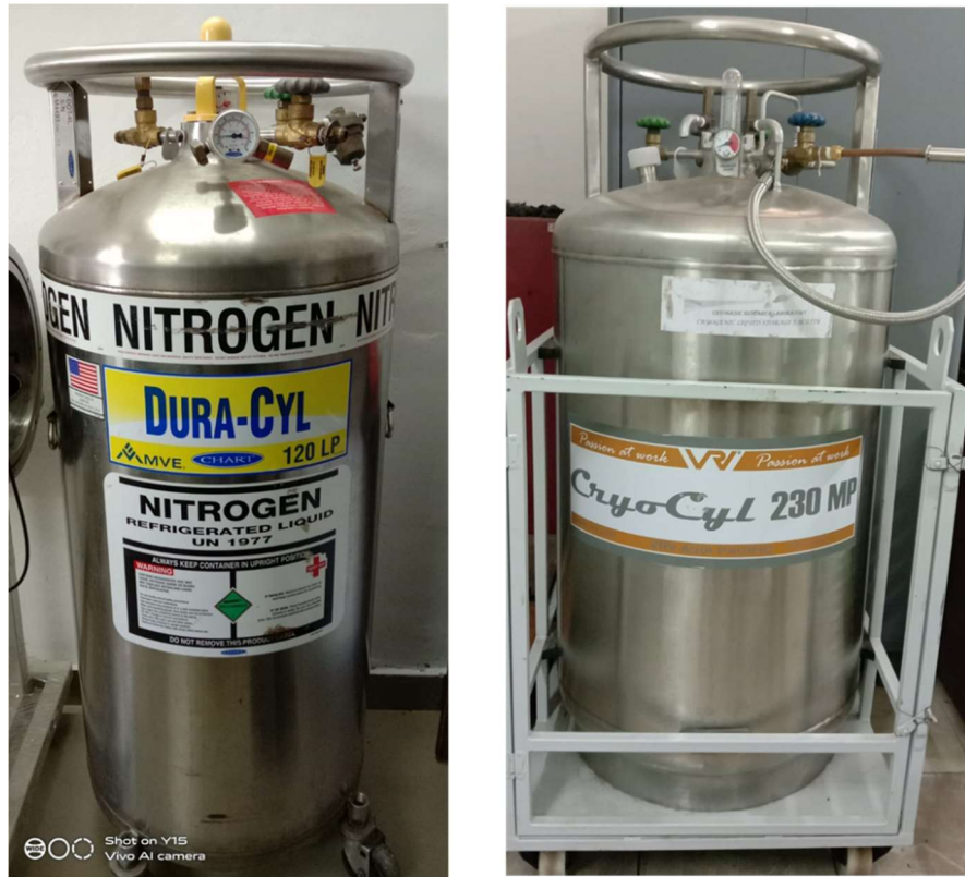
Fig: 4.23. Cryogenic storage tanks (230 L & 120 L)
