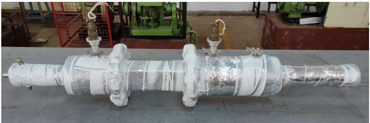
Fig: 4.19. Assembled section after applying multi-layer insulation
