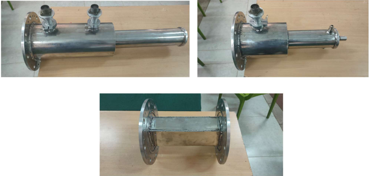
Fig: 4.17. Fabricated Inlet , Outlet & Test section
