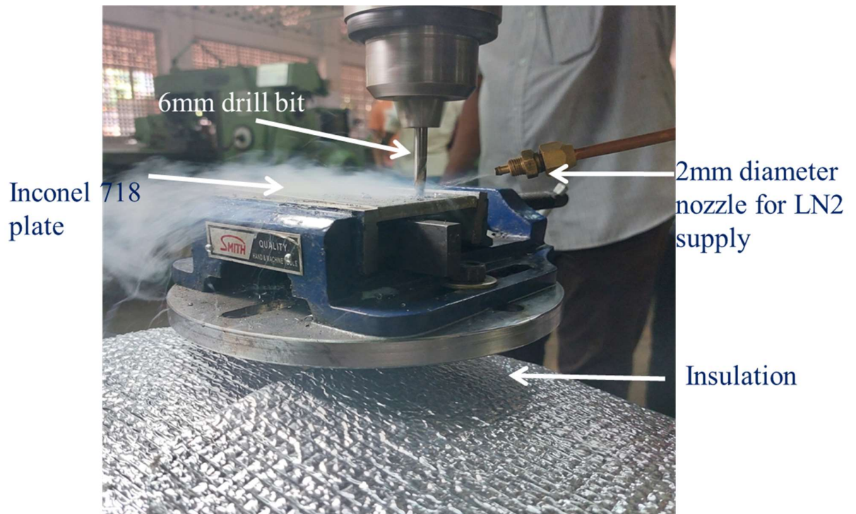
Fig 4.5. Drilling Inconel 718 using Liquid Nitrogen as coolant
