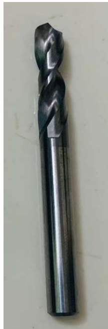
Fig. 3.4. Tungsten Carbide drill bit of 6mm diameter
