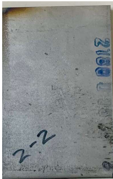
Fig. 3.3. Inconel plate of dimension 110mm*75mm*8mm
