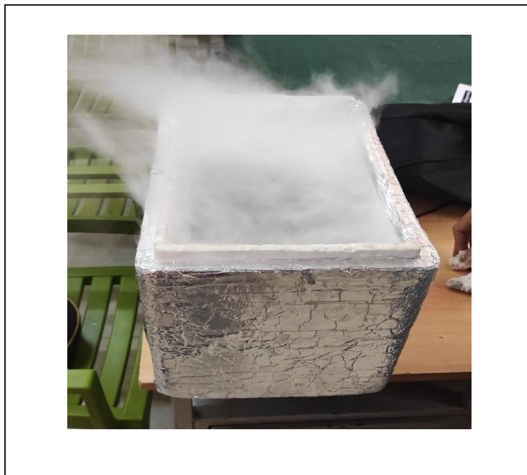
Figure-3.5 Cryogenic treatment of Hemp fiber
