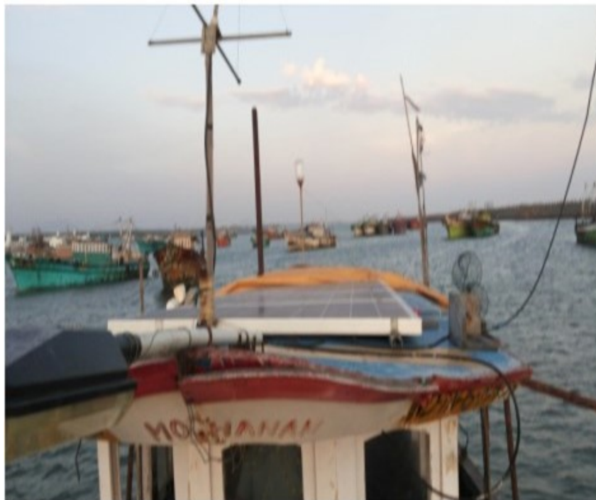
Fig. 8.1: Solar PV installed in a fishing boat
