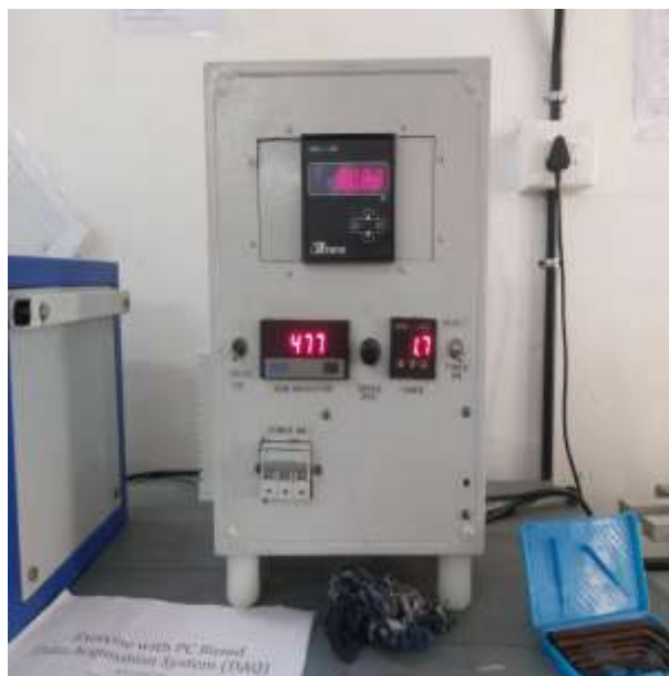
Fig 4.2 Drives with controls for rpm and time settings
