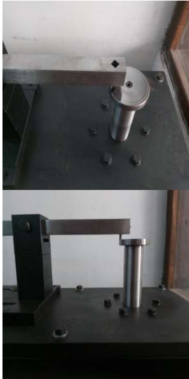
Fig 4.3 E31 Disc of diameter 65mm and Pin with diameter 6mm
