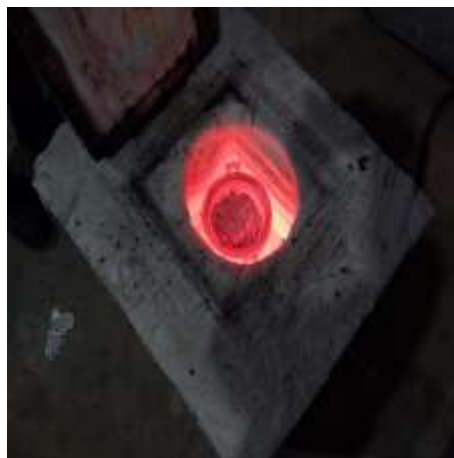
Fig 3.4 Molten aluminium in the furnace
