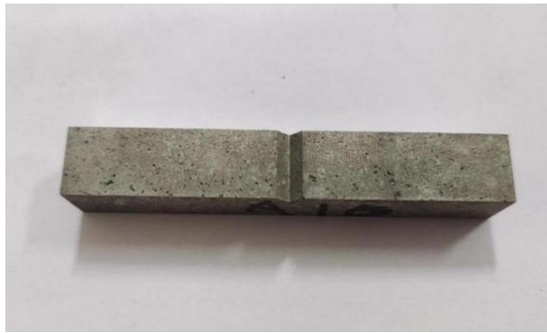
Figure 4.4 Specimen for impact testing (Top view)
