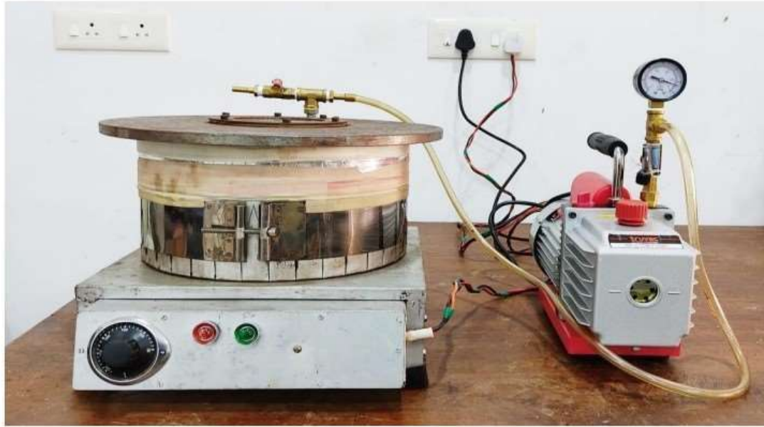
Figure 3.2: Laboratory setup of Vacuum degassing unit
