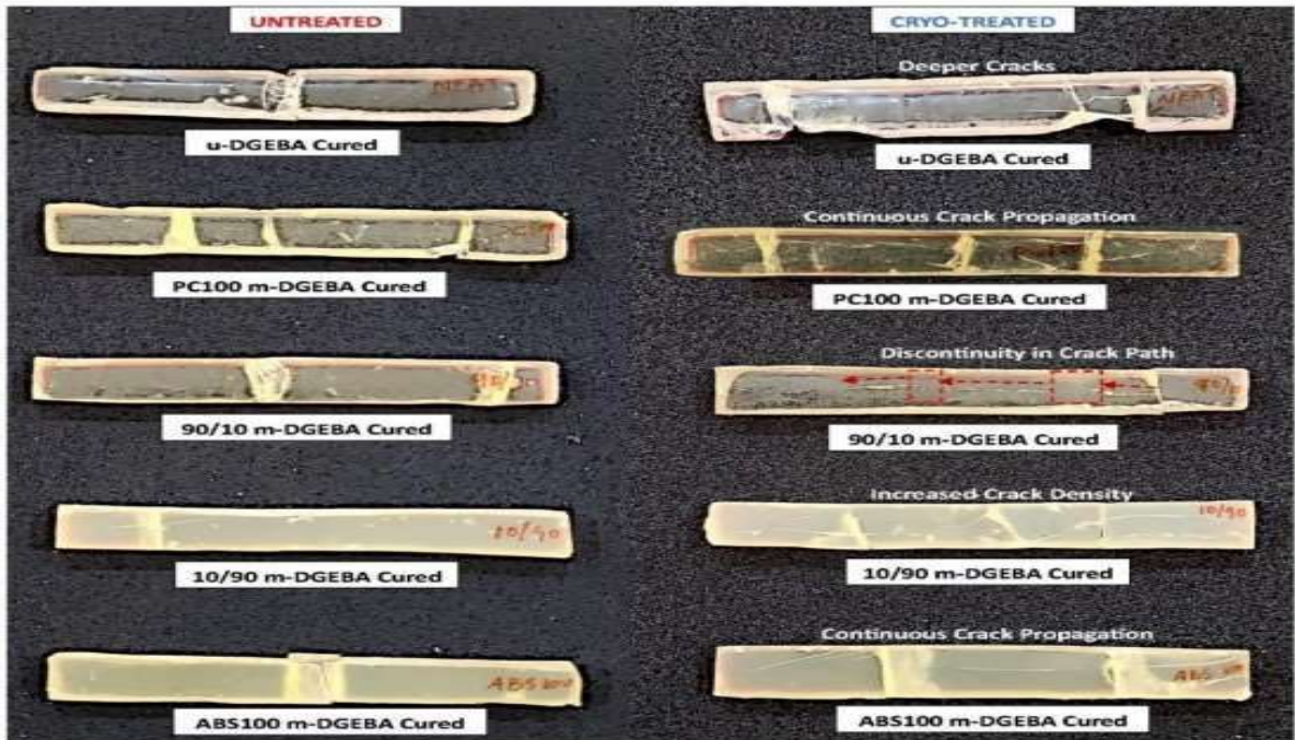
Figure 5.5: (a) Impact samples retrieved after Charpy test.
