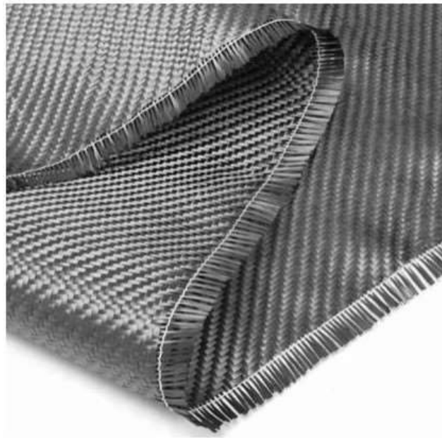
Figure 4.1: Twill weave carbon fiber
