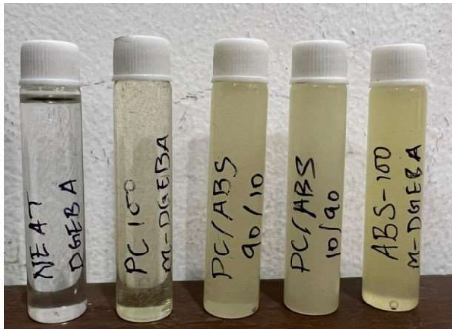
Figure 4.10: u-DEGBA and m-DGEBA resins after melt-mixing of PC/ABS blends into DGEBA at 180oC.
