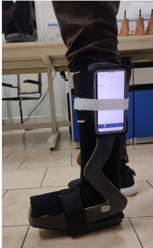
Figure 3.2 Smartphone attached to diabetic foot walker
