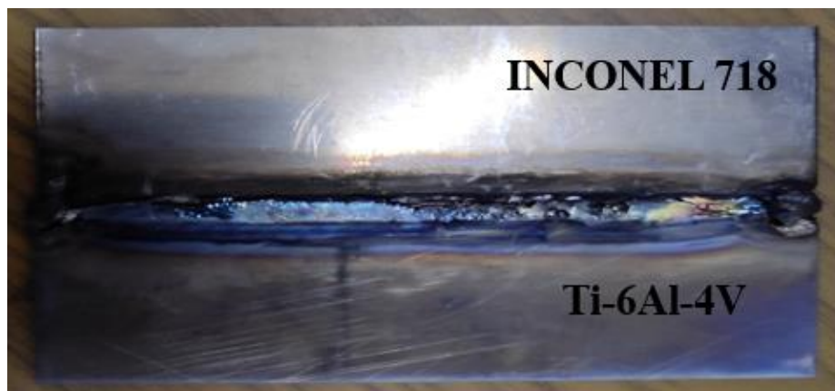
Fig 4.7: The weld generated in the presence of SiO 2 flux powder
