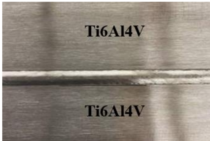
Fig 4.4: The weld joint formed between Ti6Al4V
