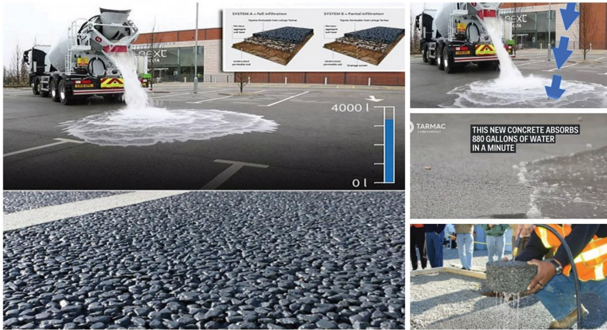
Figure 5:6: Water absorbent roads Source: (Chung, 2015)
