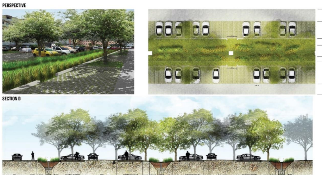
Figure 3:25 : A plan view and perspective of a re-visioned parking lot with bioswales, pervious pavement and shoreline having a vegetated bufer zone
