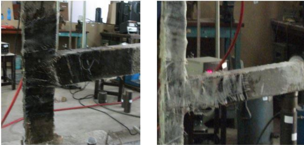
Figure 2.2 Failure of Joint after retrofitted with (a) BFRP monolithically and (b) Hybrid FRP (Source: A. Gananprangam et. al 2016)
